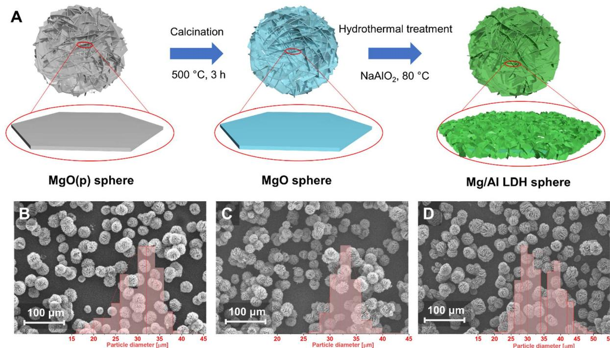
Fig. 1 (A) Schematic illustration of the synthesis of multi-hierarchical Mg/Al- $\text{CO}_3$  LDH microspheres. (B) SEM images of MgO(p) precursor spheres, (C) MgO spheres and (D) MgAl(4 h<sub>0.2</sub>) spheres (insets show the particle size distribution of the corresponding spheres measured from more than 200 particles in the SEM images by ImageJ software).
