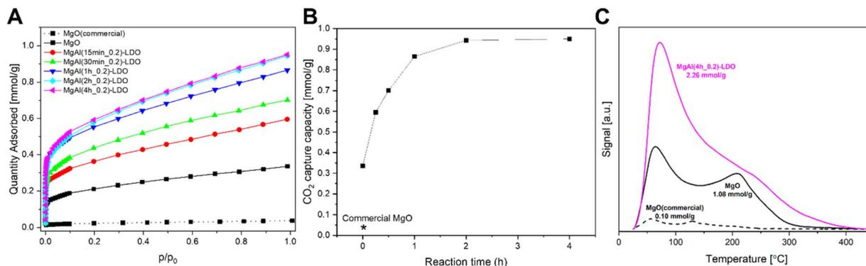
Fig. 6 (A) CO<sub>2</sub> adsorption isotherm for MgO and MgAl(x<sub>0.2</sub>)-LDO samples at 40 °C; (B) CO<sub>2</sub> capture capacity of commercial MgO and MgAl(x<sub>0.2</sub>)-LDO at 1 atm and 40 °C; (C) CO<sub>2</sub>-TPD profiles of commercial MgO, flower-like MgO microspheres and MgAl(4 h<sub>0.2</sub>)-LDO.
