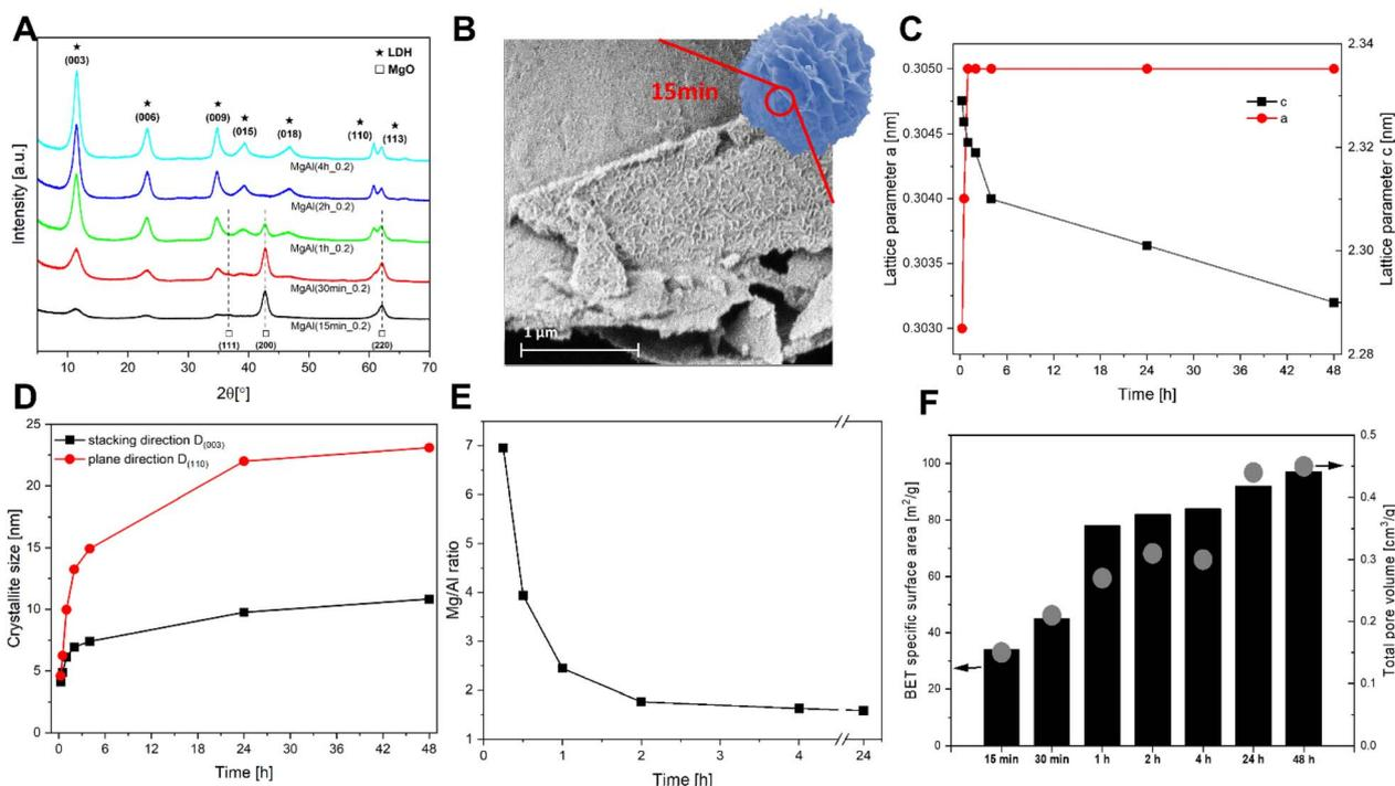
Fig. 4 A kinetic study of LDH formation from MgO microspheres at 80 °C as a function of time with Mg : Al ratio = 0.2. (A) XRD data, (B) SEM image of LDH platelets on MgAl(15 min\_0.2), (C) lattice parameters, (D) crystalline domain length, (E) Mg : Al ratio, and (F) BET specific surface area and total pore volume.
