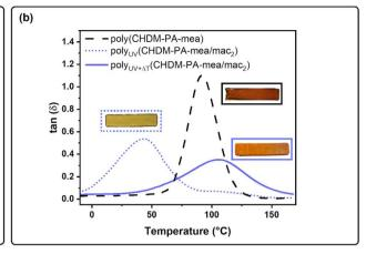
Fig. 5 (a) DSC curves of the CHDM-PA-mea precursor and poly<sub>UV</sub>(CHDM-PA-mea/mac); (b) rheology temperature sweep curves in torsion mode of poly(CHDM-PA-mea), poly<sub>UV</sub>(CHDM-PA-mea/mac<sub>2</sub>) and poly<sub>UV+AT</sub>(CHDM-PA-mea/mac<sub>2</sub>) with photos of samples tested.
