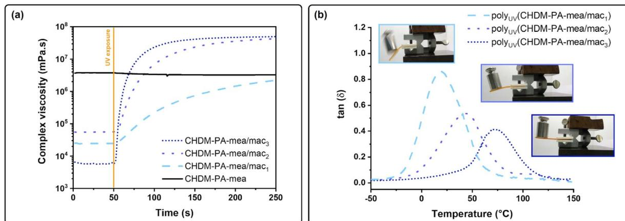
Fig. 4 (a) Isothermal UV rheokinetic measurements of CHDM-PA-mea/mac monomers at room temperature; (b) rheology temperature sweep curves in torsion mode of poly<sub>UV</sub>(CHDM-PA-mea/mac) materials and photos of sample bending (room temperature).
