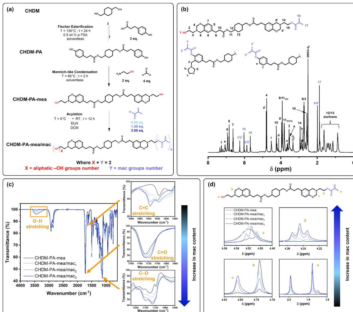
Fig. 2 (a) Synthetic route for photopolymerisable benzoxazine precursors; (b)  $^1\text{H}$  NMR spectrum of the main structure of CHDM-PA-mea/mac<sub>2</sub> precursor and related substructures; (c) FTIR spectra of CHDM-PA-mea and CHDM-PA-mea/mac precursors highlighting characteristic peaks (simplified spectra; see full spectra in Fig. S20†); (d) focus on regions of  $^1\text{H}$  NMR spectra of CHDM-PA-mea and CHDM-PA-mea/mac precursors (simplified spectra; see full spectra in Fig. S18†).
