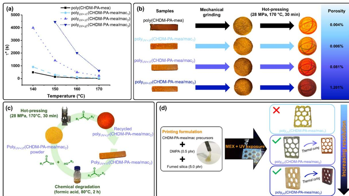
Fig. 6 (a) Evolution of relaxation times of each  $\text{poly}_{\text{UV}+\Delta T}(\text{CHDM-PA-mea/mac})$  composition as a function of temperature; (b) photographs of the mechanical recycling of  $\text{poly}_{\text{UV}+\Delta T}(\text{CHDM-PA-mea/mac})$ ; (c) chemical recycling strategy adopted for  $\text{poly}_{\text{UV}+\Delta T}(\text{CHDM-PA-mea/mac}_2)$ ; (d) photographs of honeycombs obtained after 3D printing trials by MEX with CHDM-PA-mea/mac precursor based formulations.
