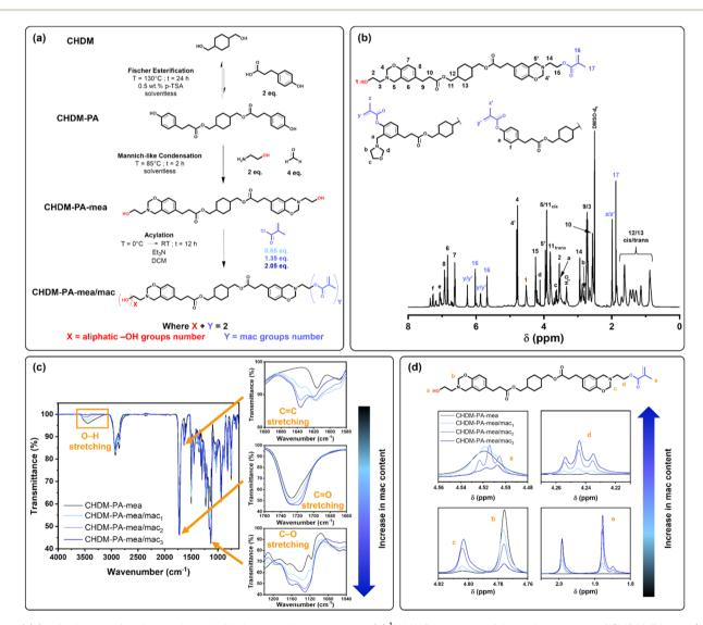
Fig. 2 (a) Synthetic route for photopolymerisable benzoxazine precursors; (b) <sup>1</sup>H NMR spectrum of the main structure of CHDM-PA-mea/mac<sub>2</sub> precursor and related substructures; (c) FTIR spectra of CHDM-PA-mea and CHDM-PA-mea/mac precursors highlighting characteristic peaks (simplified spectra; see full spectra in Fig. S20†); (d) focus on regions of <sup>1</sup>H NMR spectra of CHDM-PA-mea and CHDM-PA-mea/mac precursors (simplified spectra; see full spectra in Fig. S18†).
