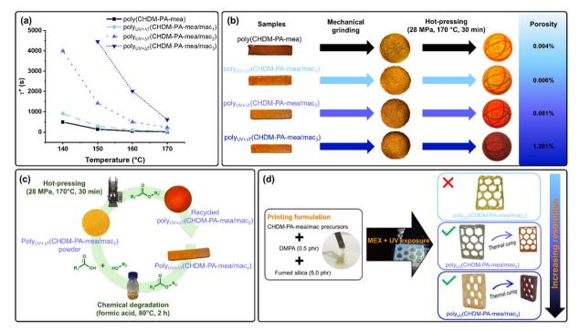
Fig. 6 (a) Evolution of relaxation times of each poly $_{UV+\Delta T}$  (CHDM-PA-mea/mac) composition as a function of temperature; (b) photographs of the mechanical recycling of poly<sub>UV+ $\Delta T$ </sub>(CHDM-PA-mea/mac); (c) chemical recycling strategy adopted for poly<sub>UV+ $\Delta T$ </sub>(CHDM-PA-mea/mac<sub>2</sub>); (d) photographs of honeycombs obtained after 3D printing trials by MEX with CHDM-PA-mea/mac precursor based formulations
