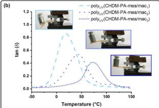
Fig. 4 (a) Isothermal UV rheokinetic measurements of CHDM-PA-mea/mac monomers at room temperature; (b) rheology temperature sweep curves in torsion mode of poly<sub>UV</sub>(CHDM-PA-mea/mac) materials and photos of sample bending (room temperature).
