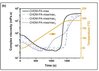
Fig. 3 (a) DSC curves and (b) rheokinetic measurements of CHDM-PA-mea and CHDM-PA-mea/mac monomers.
