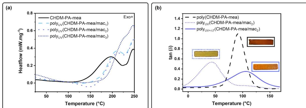
Fig. 5 (a) DSC curves of the CHDM-PA-mea precursor and poly<sub>UV</sub>(CHDM-PA-mea/mac); (b) rheology temperature sweep curves in torsion mode of poly(CHDM-PA-mea), poly<sub>UV</sub>(CHDM-PA-mea/mac<sub>2</sub>) and poly<sub>UV+ΔT</sub>(CHDM-PA-mea/mac<sub>2</sub>) with photos of samples tested.
