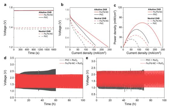
Fig. 6 (a) Open-circuit voltage, (b) discharge polarization curves, and (c) power density curves of alkaline ZABs and neutral ZABs. Long-term discharge/charge cycling tests of (d) alkaline ZABs at 5 mA cm<sup>-2</sup> with each cycle for 20 min and (e) neutral ZABs at 2.5 mA cm<sup>-2</sup> with each cycle for 20 min, using Fe,Pd-NC + RuO<sub>2</sub> and Pt/C + RuO<sub>2</sub> catalysts.
