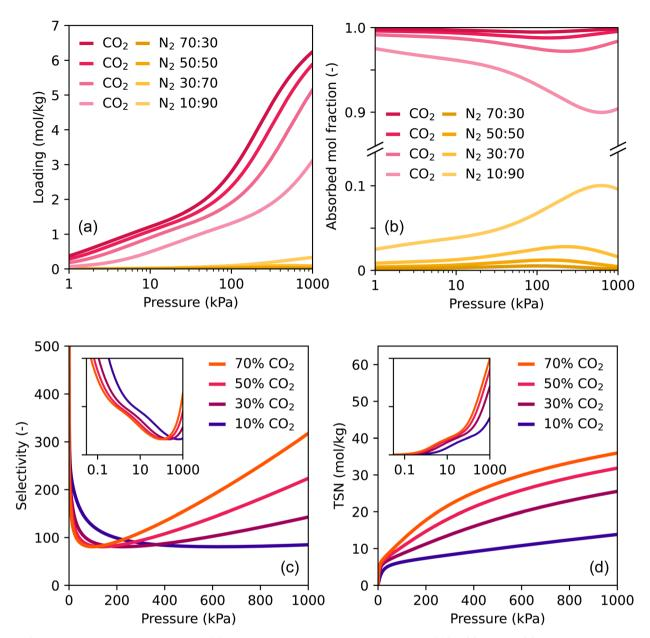
Fig. 4 IAST predictions of the adsorption from CO<sub>2</sub>: N<sub>2</sub>-mixtures of four bulk compositions at 298 K. (a) Loading, (b) adsorbed mole fraction, (c) selectivity and (d) trade-off between selectivity and uptake (TSN, see Methodology). The insets show the selectivity and TSN plotted in logarithmic scale.
