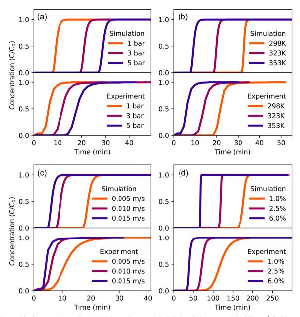
Fig. 5 Simulated (top) and experimental (bottom) breakthrough curves of  $CO_2$  in helium. (a) Pressures at 353 K, 0.01 m s<sup>-1</sup>, 6% (b) temperatures at 1 bar,  $0.01 \,\mathrm{m\,s^{-1}}$ , 6% (c) velocities at 353 K, 1 bar, 6% (d) concentrations at 298 K, 1 bar,  $0.005 \,\mathrm{m\,s^{-1}}$ .  $C_0$  is the CO<sub>2</sub>-concentration at the inlet.
