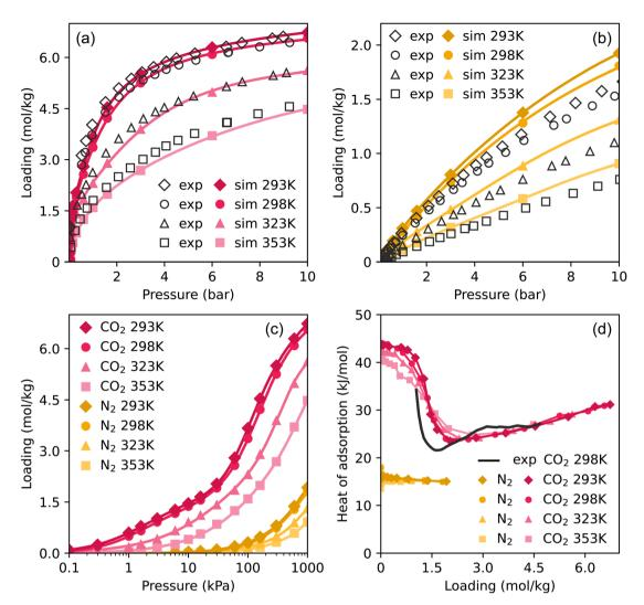
Fig. 2 Experimental and simulated adsorption isotherms of (a)  $CO_2$  and (b)  $N_2$  at four temperatures. The colored points are the results of the MC-simulations and the drawn curves are the fitted isotherms. Simulated (c) isotherms and (d) heats of adsorption of  $CO_2$  and  $N_2$ . The simulated heats of adsorption are computed using a fluctuation formula.<sup>38</sup>
