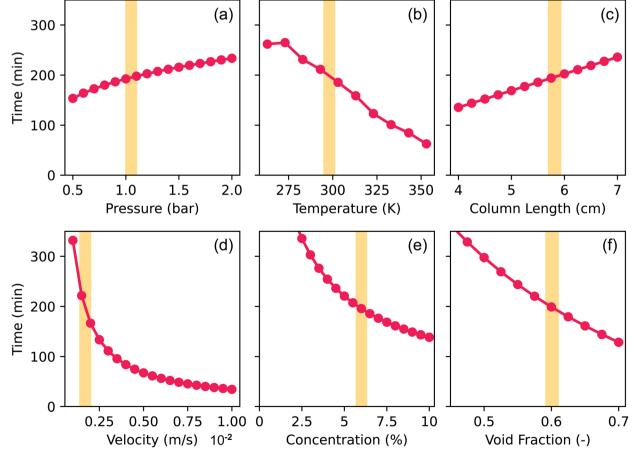
Fig. 7 Time where equilibrium ( $C/C_0 = 1$ ) of CO<sub>2</sub> is reached in the modeling of the breakthrough curves of CO<sub>2</sub> and N<sub>2</sub> in TAMOF-1. The (a) pressure, (b) temperature, (c) column length, (d) gas velocity, (e) CO<sub>2</sub>-concentration and (f) void fraction are varied, while keeping the other conditions fixed at the conditions of the experiment shown in Fig. 6 (shown with the yellow bands and listed in Table S7†).
