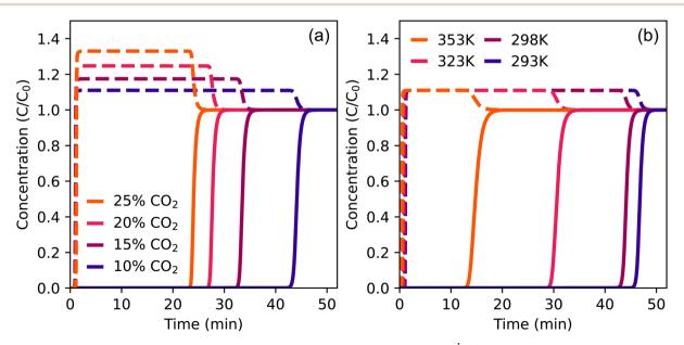
Fig. 8 Simulated breakthrough curves of  $CO_2$  (solid) and  $N_2$  (dashed) at 1 bar and 0.005 m s<sup>-1</sup>. (a) Different concentrations of  $CO_2$  at 298 K (b) different temperatures of 10% CO<sub>2</sub>.
