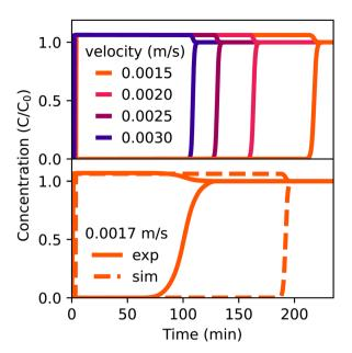
Fig. 6 Bottom: simulated and experimental breakthrough curves of  $6\% \text{ CO}_2$  and  $94\% \text{ N}_2$  at 298 K, 1 bar and  $0.0017 \text{ m s}^{-1}$ . Top: simulated curves with same conditions at different initial velocities. The retained curves is in all cases  $\text{CO}_2$ ,  $\text{N}_2$  leaves the column almost immediately.
