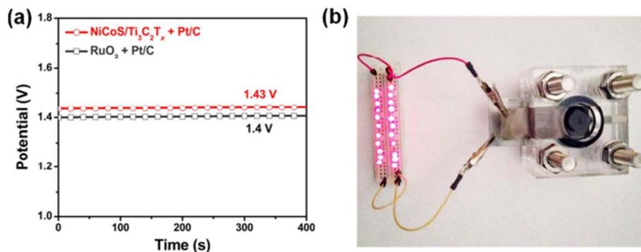
Fig. 30 (a) Open-circuit voltage plots for rechargeable Zn–air batteries with NiCoS/Ti<sub>3</sub>C<sub>2</sub>T<sub>x</sub> + Pt/C and RuO<sub>2</sub> + Pt/C configurations. (b) Red LED array powered by a Zn–air battery using NiCoS/Ti<sub>3</sub>C<sub>2</sub>T<sub>x</sub> + Pt/C air cathode. Reproduced from ref. 133 with permission from American Chemical Society, copyright © 2018.
