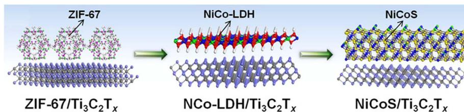
Fig. 29 Diagram of the preparation process for  $\text{NiCoS}/\text{Ti}_3\text{C}_2\text{T}_x$ . Reproduced from ref. 133 with permission from American Chemical Society, copyright © 2018.
