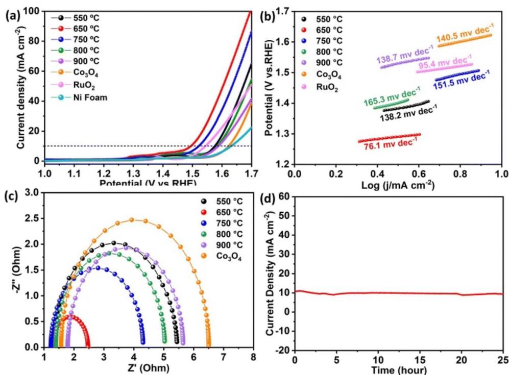
Fig. 24 (a) Polarization graphs for  $\text{CoTiO}_x\text{-T}$  samples and  $\text{Co}_3\text{O}_4$ -coated Ni foam. (b) Tafel diagrams for these catalysts. (c) Nyquist diagrams. (d) Temporal amperometry of  $\text{CoTiO}_x\text{-650}$  at 1.49 V versus RHE. Reproduced from ref. 108 with permission from Royal Society of Chemistry, copyright © 2023.
