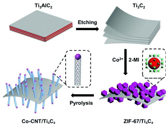
Fig. 17 Schematic illustration of the formation process for Co-CNT/Ti<sub>3</sub>C<sub>2</sub> composites. Reproduced from ref. 91 with permission from Royal Society of Chemistry, copyright © 2024.
