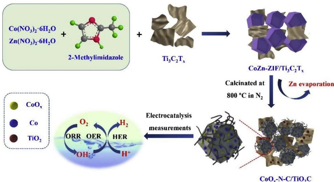
Fig. 22 Diagram illustrates the preparation process for the CoO<sub>x</sub>-N-C/TiO<sub>2</sub>C catalyst.<sup>97</sup> Reproduced from ref. 97 with permission from Elsevier Ltd, copyright © 2019.
