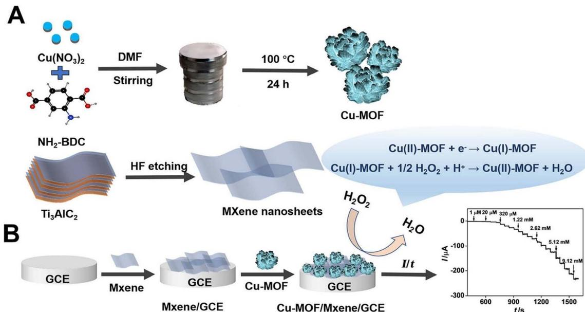
Fig. 8 (A) Synthesis of 3D flower-like Cu-MOF and ultra-thin MXene nanosheets. (B) Construction of an electrochemical sensor for  $\text{H}_2\text{O}_2$  detection. Reproduced from ref. 66 with permission from Wiley, copyright © 2021.
