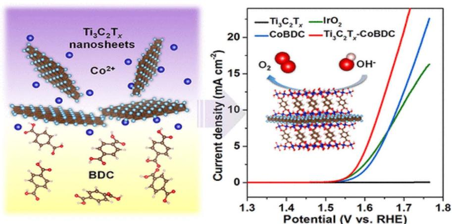
Fig. 31 Schematic of Ti<sub>3</sub>C<sub>2</sub>T<sub>x</sub>–CoBDC hybrid preparation for the oxygen evolution reaction, with OER polarization curves. Reproduced from ref. 141 with permission from American Chemical Society, copyright © 2017.
