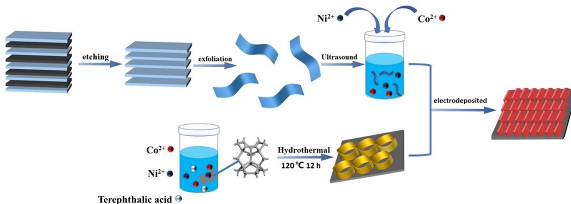
Fig. 10 Schematic of the fabrication process for the M-NC@NCM/NF electrode. Reproduced from ref. 73 with permission from Elsevier, copyright © 2021.
