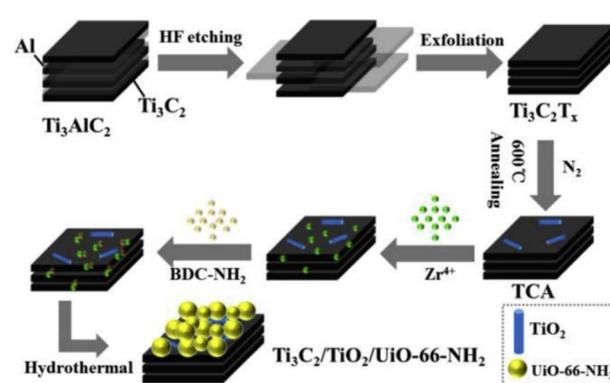
Fig. 4 Schematic of the reaction route for forming Ti<sub>3</sub>C<sub>2</sub>/TiO<sub>2</sub>/UiO-66-NH<sub>2</sub>.<sup>54</sup> Reproduced from ref. 54 with permission from Elsevier Ltd, copyright © 2019.
