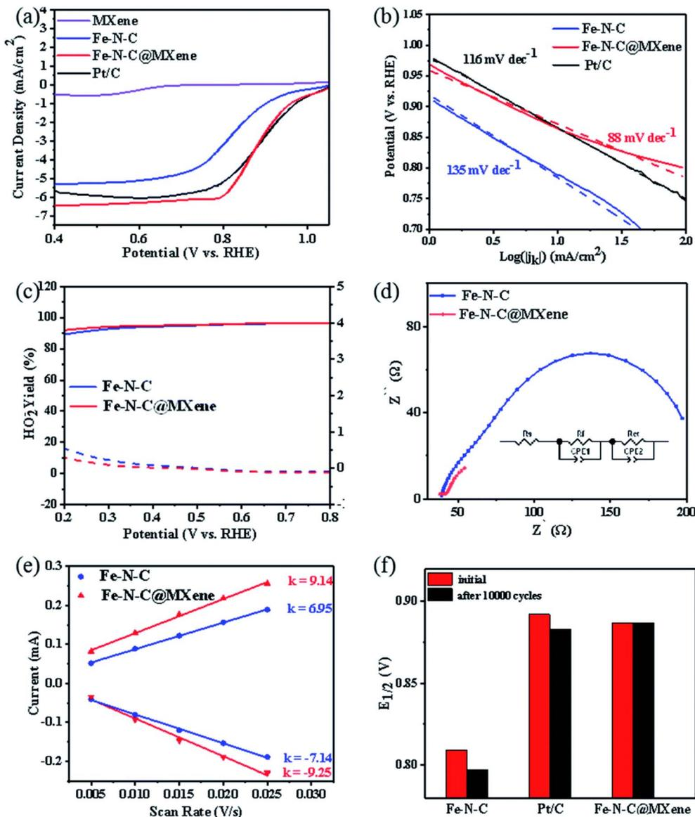
Fig. 14 (a) Linear sweep voltammograms for MXene, Fe-N-C, Fe-N-C@MXene, and Pt/C; (b) linear sweep potentials for Fe-N-C, Fe-N-C@MXene, and Pt/C; (c) ETR and  $\text{HO}_2^-$  production for Fe-N-C and Fe-N-C@MXene; (d) electrochemical impedance spectroscopy and schematic representation; (e) voltage vs. scan rate for Fe-N-C and Fe-N-C@MXene; (f) electrochemical stability of Fe-N-C, Fe-N-C@MXene, and Pt/C. Reproduced from ref. 83 with permission from Royal Society of Chemistry, copyright © 2021.
