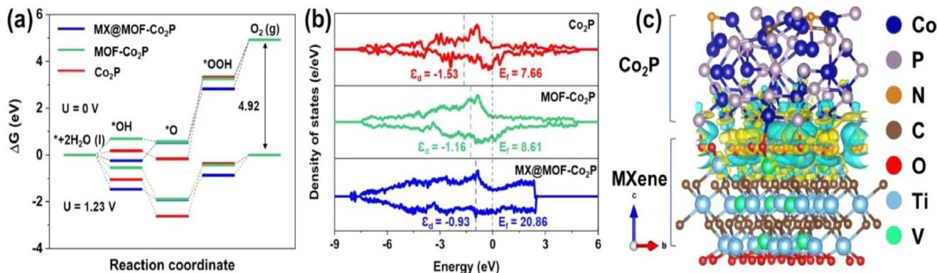
Fig. 25 (a) Energy flow chart for open educational resources. (b) Distribution of charge density (DOS) along with the associated d-band center and Fermi energy ( $E_f$ ). (c) Charge density difference across the  $\text{Co}_2\text{P}$ –MXene boundary, with yellow showing electron gathering and blue showing electron shedding. Reproduced from ref. 114 with permission from Elsevier Ltd, copyright © 2023.
