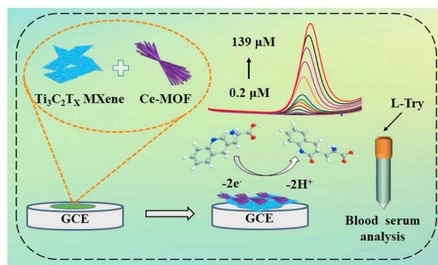
Fig. 7 Schematic illustrating the fast production method for a three-dimensional Ce-MOF/ $\text{Ti}_3\text{C}_2\text{T}_x$  MXene blend aimed at achieving superior electrochemical sensing of L-tryptophan. Reproduced from ref. 65 with permission from Elsevier Ltd, copyright © 2022.
