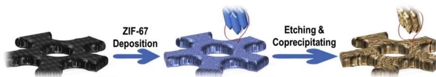
Fig. 26 Schematic of the synthesis process for  $\text{CoFe MLDH/Ti}_3\text{C}_2$ . Reproduced from ref. 126 with permission from Elsevier Ltd, copyright © 2021.
