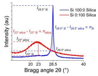
Fig. 3 XRD diffractograms of pure Si and SiO<sub>2</sub>, and the use of peak intensities of both taken at 23° and 28.5° for calculating the peak intensity ratio (PIR).
