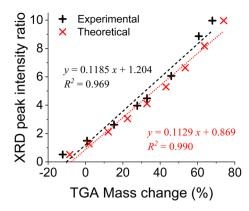
Fig. 5 A comparison between TGA-based and XRD-based results obtained from both theoretical calibrations and measurements of real mixtures of silica and silicon.
