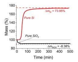
Fig. 1  $\,$  TGA of pure Si (50 nm) and SiO<sub>2</sub> (Sorbosil), conducted in air.
