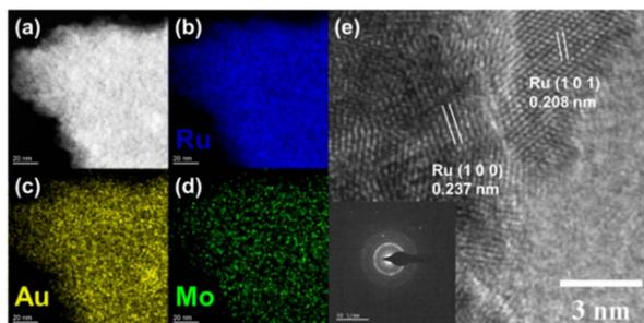
Fig. 2 TEM images of the RuAu-2MoO<sub>x</sub> deposit: (a–d) images of elemental mapping and (e) corresponding images of the RuAu-2MoO<sub>x</sub> deposit. The insets show a selected-area electron diffraction pattern of (e).
