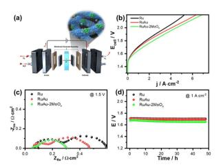
Fig. 6 Electrochemical measurements for Ru, RuAu, and RuAu- $2\text{MoO}_x$  as the electrocatalyst for the HER in PEMWE. (a) Schematic diagram of the PEMWE unit cell with the RuAu- $\text{MoO}_x$  electrocatalyst. (b) j-V curves of the PEMWE cell. (c) Nyquist plots with an amplitude of 18 mV and an applied voltage of 1.5 V. (d) Chronopotentiometry response at a current density of 1A cm<sup>-2</sup> during 48 hours of operation.
