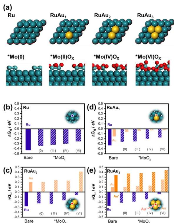
Fig. 5 (a) Atomic structures of RuAu surfaces with varying Au content and adsorbed  $\text{MoO}_x$  clusters with different oxidation states. H-binding free energies ( $\Delta G_{\text{H}}$ ) for various active sites on (b) Ru, (c) RuAu<sub>1</sub>, (d) RuAu<sub>2</sub>, and (e) RuAu<sub>3</sub> surfaces with and without  $\text{MoO}_x$  clusters. Blue bars represent Ru sites, orange bars represent Au sites, and hatched bars indicate sites affected by  $\text{MoO}_x$ .
