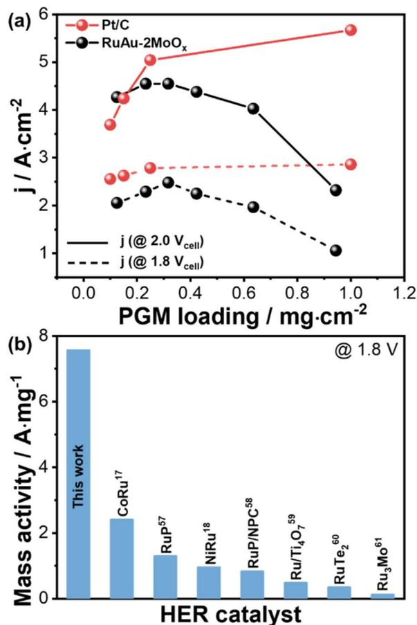
Fig. 7 (a) The performance of PEMWE cells loaded with RuAu-2MoO<sub>x</sub> or Pt/C at the cell voltages of 1.8 and 2.0 V with various catalyst loading amounts. (b) The comparison of the performance at 1.8 V with values reported in the literature dealing with Ru-related HER electrocatalysts.
