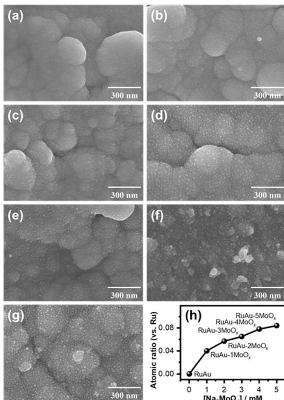
Fig. 1 Top view SEM images of (a) Ru, (b) RuAu, and (c–g) RuAu-1–5MoO<sub>x</sub> deposits on Ti foil. (h) Plot of the atomic ratio of Mo to Ru.
