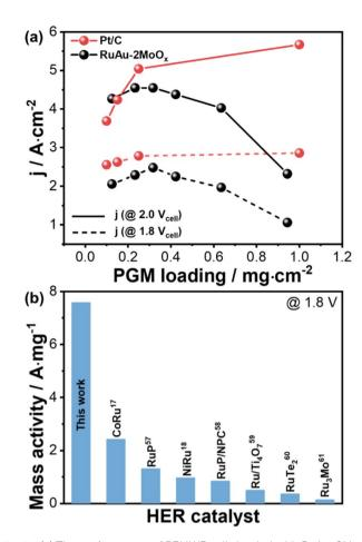
Fig. 7 (a) The performance of PEMWE cells loaded with RuAu- $2MoO_x$  or Pt/C at the cell voltages of 1.8 and 2.0 V with various catalyst loading amounts. (b) The comparison of the performance at 1.8 V with values reported in the literature dealing with Ru-related HER electrocatalysts.
