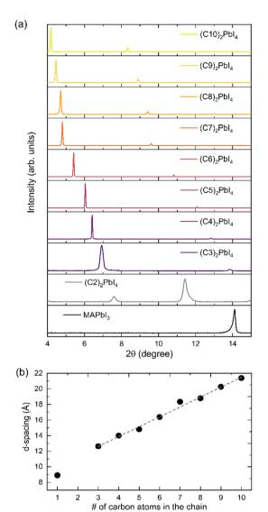
Fig. 1 Structural analysis of the perovskite films. (a) XRD patterns of 2D perovskite and MAPbI<sub>3</sub> with different A-site cations in the range of  $2\theta$ from 4° to 15°. A wider region is shown in Fig. S5 in the ESI.† (b) Extracted relationship between the number of the carbon atoms in the spacer cation and the resulting d-spacing of the perovskite film; note that the C1 sample corresponds to the 3D perovskite MAPbI<sub>3</sub>.
