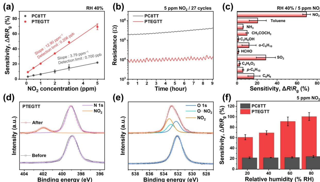
Fig. 5 NO<sub>2</sub> chemiresistors. (a) Sensitivity upon exposure to 0.1–5 ppm NO<sub>2</sub> using the CPs. (b) Resistance changes under cycling NO<sub>2</sub> exposure. (c) Selective sensing properties towards various analytes. XPS profiles of PTEGTT: (d) N 1s and (e) O 1s. (f) Sensitivity depending on relative humidity (RH).
