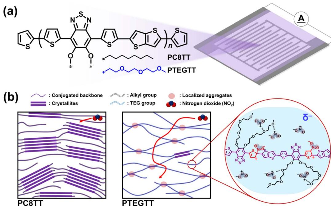
Fig. 1 (a) Chemical structure of the CPs for chemiresistors. (b) Schematic illustrations of the polymer morphologies and NO<sub>2</sub> behavior in the CPs.
