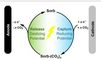
Fig. 1 Schematic of an electro-swing carbon capture system.
