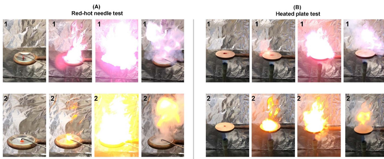
Fig. 11 (A) Hot needle test of 1 and 2. (B) Hot plate test of 1 and 2.
