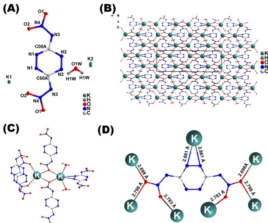
Fig. 4 (A) Labeling scheme for  $1 \cdot \text{H}_2\text{O}$  (thermal ellipsoid at 50%). (B) Crystal packing of 1. (C and D) Coordination modes of  $\text{K}^+$ .
