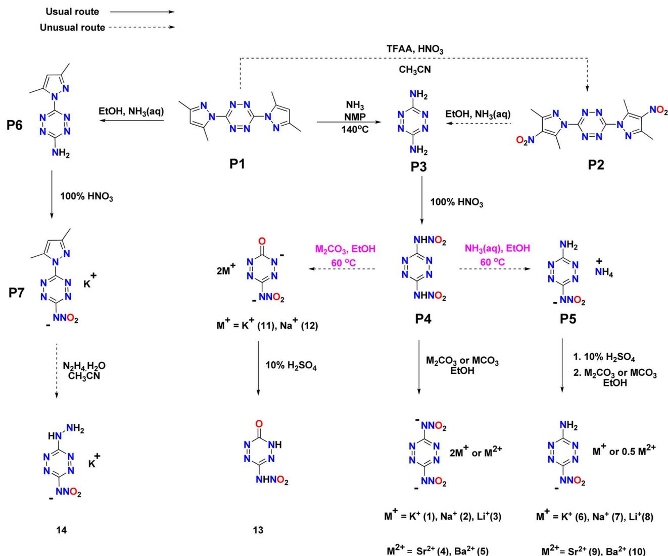
Scheme 1 Reactions of 3,6-bis(3,5-dimethyl-1H-pyrazol-1-yl)-1,2,4,5-tetrazine (P1) and temperature-based reactivity of *N,N'*-(1,2,4,5-tetrazine-3,6-diyl)dinitramide (P4).
