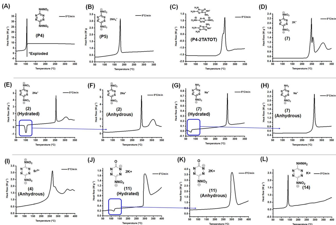
Fig. 9 Differential scanning calorimetry (DSC) analysis (A) P4. (B) P5. (C) P4-2TATOT. (D) **7**. (E) **2**-Hydrated. (F) **2**-Anhydrous. (G) **7**-Hydrated. (H) **7**-Anhydrous. (I) **4**-Anhydrous. (J) **11**-Hydrated. (K) **11**-Anhydrous. (L) **14**.
