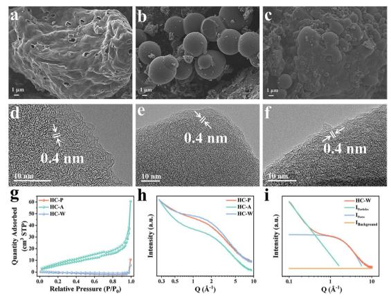
Fig. 2 SEM images of (a) HC-P, (b) HC-A, and (c) HC-W. TEM images of (d) HC-P, (e) HC-A, and (f) HC-W. (g)  $N_2$  adsorption—desorption isotherms and (h) SAXS patterns of HC-P, HC-A and HC-W. (i) Fitted SAXS pattern of HC-W.
