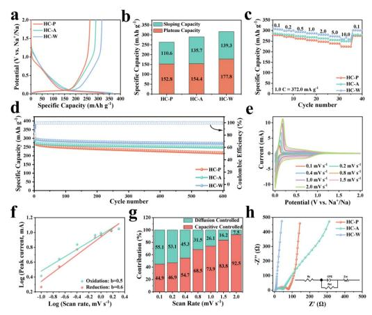
Fig. 4 (a) The initial discharge/charge curves of HC-P, HC-A and HC-W at 0.1C. (b) Discharge capacity contributions from the slope region and plateau region. (c) Rate performance of HC-P, HC-A and HC-W. (d) Cycling stability of HC-P, HC-A and HC-W at 1.0C for 600 cycles. (e) CV curves at different scan rates from 0.1 to 2.0 mV s<sup>-1</sup> and (f) b-values of HC-W. (g) Capacitive contributions at different scan rates of HC-W. (h) Nyquist plots in the initial state.
