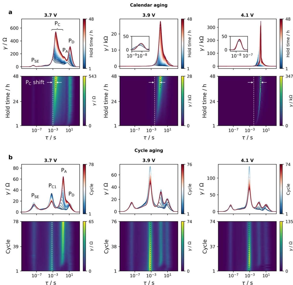
Fig. 5 DRT evolution and corresponding 2D DRT surfaces (a) during potentiostatic hold and (b) at end of discharge of cycles in high C-rate regime. In 2D DRT, the maximum value displayed on each color bar represents approximately the highest DRT intensity and the dashed lines indicate the relative position of  $P_C$  peak. Data from all investigated cut-offs with Nyquist and Bode plots can be found in Fig. S6–S9.†
