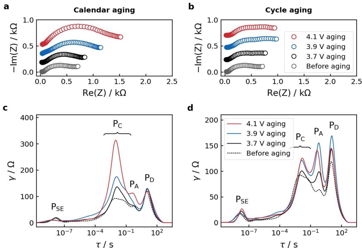
Fig. 6 Data measured at the last formation cycles (before aging) and last RPT cycles (aging). (a and b) Nyquist plots and (c and d) DRT of calendar and cycle aging cells, respectively. Data from all investigated cut-offs can be found in Fig. S10.†
