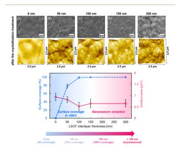
Fig. 2 Surface SEM and AFM images: (a and f) 0 nm, (b and g) 50 nm, (c and h) 100 nm, (d and i) 150 nm, and (e and j) 300 nm  $La_{0.6}Sr_{0.4}$ - $Co_{0.4}Fe_{0.6}O_{3-\delta}$  (LSCF) interlayer. (k) Comparison of surface coverage and surface area as a function of LSCF interlayer thickness, demonstrating the morphological evolution of the LSCF interlayer on the samaria-doped ceria electrolyte sintered at 900 °C for 2 h (after heat treatment)
