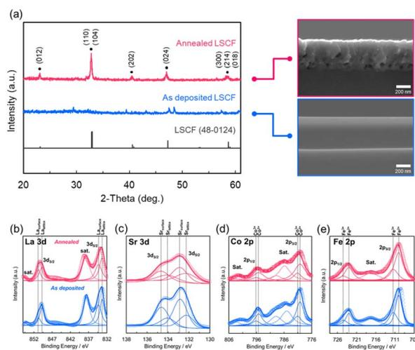
Fig. 1 (a) XRD survey spectra and cross-sectional SEM images and XPS spectra of (b) La 3d, (c) Sr 3d, (d) Co 2p, and (e) Fe 2p of the  $\text{La}_{0.6}\text{-Sr}_{0.4}\text{Co}_{0.4}\text{Fe}_{0.6}\text{O}_{3-\delta}$  (LSCF) interlayer, as deposited and annealed at 900 °C for 2 h on a Si (100) wafer.
