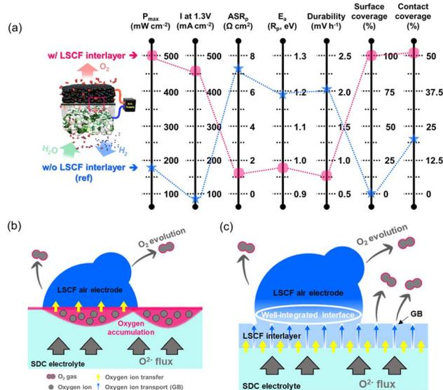
Fig. 7 (a) Comparison of the structural characteristics and electrochemical performances. Schematic illustrations of the proposed reaction mechanisms: (b) reference (w/o the LSCF interlayer) and (c) modified (w/o the LSCF interlayer) samples.
