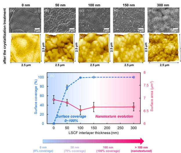
Fig. 2 Surface SEM and AFM images: (a and f) 0 nm, (b and g) 50 nm, (c and h) 100 nm, (d and i) 150 nm, and (e and j) 300 nm  $\text{La}_{0.6}\text{Sr}_{0.4}\text{-Co}_{0.4}\text{Fe}_{0.6}\text{O}_{3-\delta}$  (LSCF) interlayer. (k) Comparison of surface coverage and surface area as a function of LSCF interlayer thickness, demonstrating the morphological evolution of the LSCF interlayer on the samaria-doped ceria electrolyte sintered at 900 °C for 2 h (after heat treatment).
