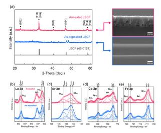
Fig. 1 (a) XRD survey spectra and cross-sectional SEM images and XPS spectra of (b) La 3d, (c) Sr 3d, (d) Co 2p, and (e) Fe 2p of the La<sub>0.6</sub>- $Sr_{0.4}Co_{0.4}Fe_{0.6}O_{3-\delta}$  (LSCF) interlayer, as deposited and annealed at 900 °C for 2 h on a Si (100) wafer.
