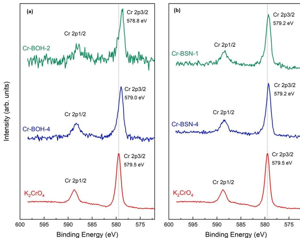
Fig. 9 Cr 2p XPS spectra for (a) BOH exposed to 1040 ppm Cr (0.02 M; sample S) in Hanford SGW (Cr-BOH-2) and DIW (Cr-BOH-4) and (b) BSN exposed to 1040 ppm Cr in Hanford SGW (Cr-BSN-1) and DIW (Cr-BSN-4) for 24 hours.
