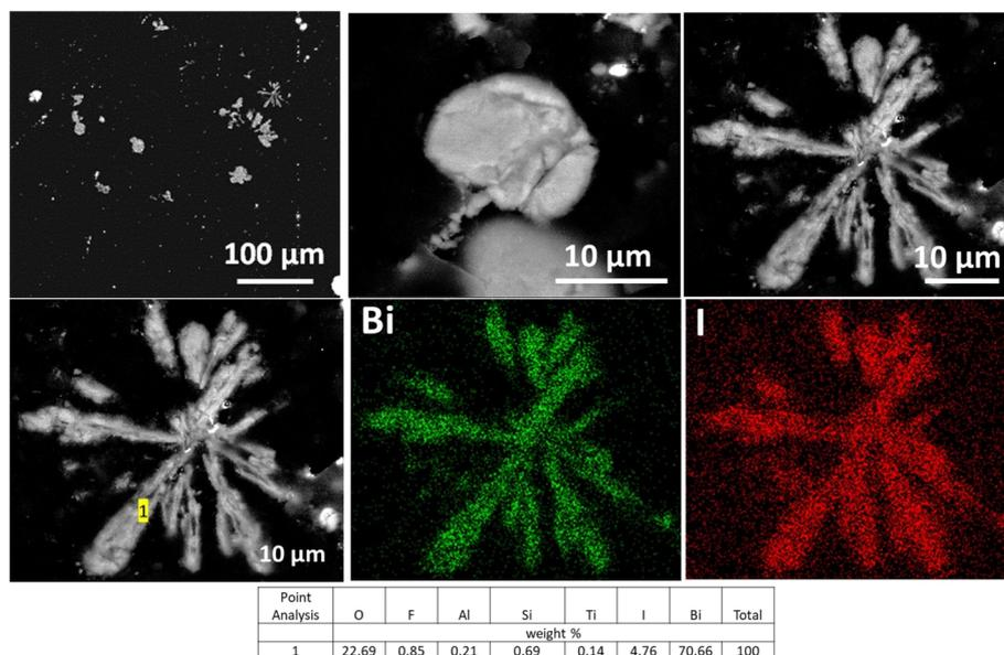
Fig. 15 SEM images and EDS maps for BOH exposed to 190 ppm I (1.5 mM; sample E) in Hanford SGW for 24 hours.
