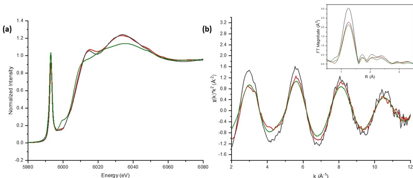
Fig. 8 (a) Cr K-edge XANES spectra; (b)  $k^2$ -weighted  $\chi(k)$  spectra and Fourier transform magnitude for Cr (1040 ppm or 0.02 M; sample S) associated with BOH (black line), BSN (red line) and for a 1.45 molal solution of  $\text{CrO}_4^{2-}$  at pH 13 (green line).<sup>39</sup>
