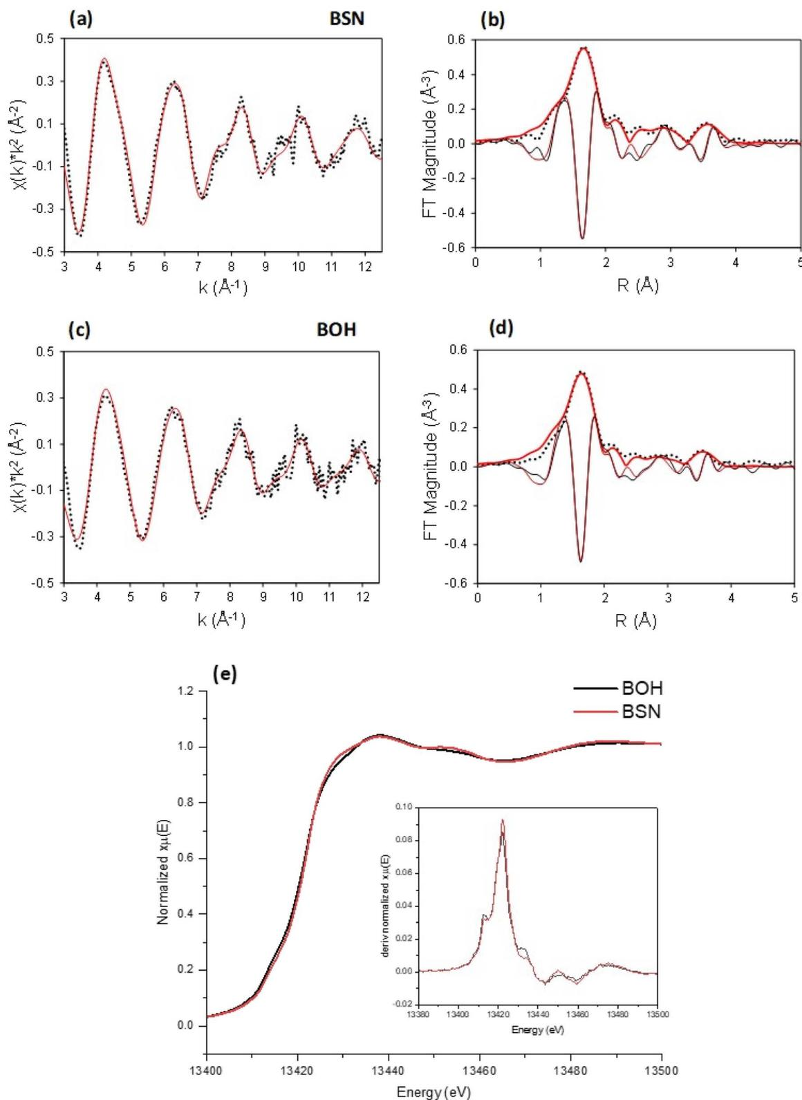
Fig. 2 Bi L<sub>III</sub>-edge XAS for BSN and BOH. (a) EXAFS and (b) transform magnitude with imaginary part for BSN; (c) EXAFS and (d) transform magnitude with imaginary part for BOH. (e) XANES for BOH and BSN starting materials with the inset of derivatives of normalized absorption.
