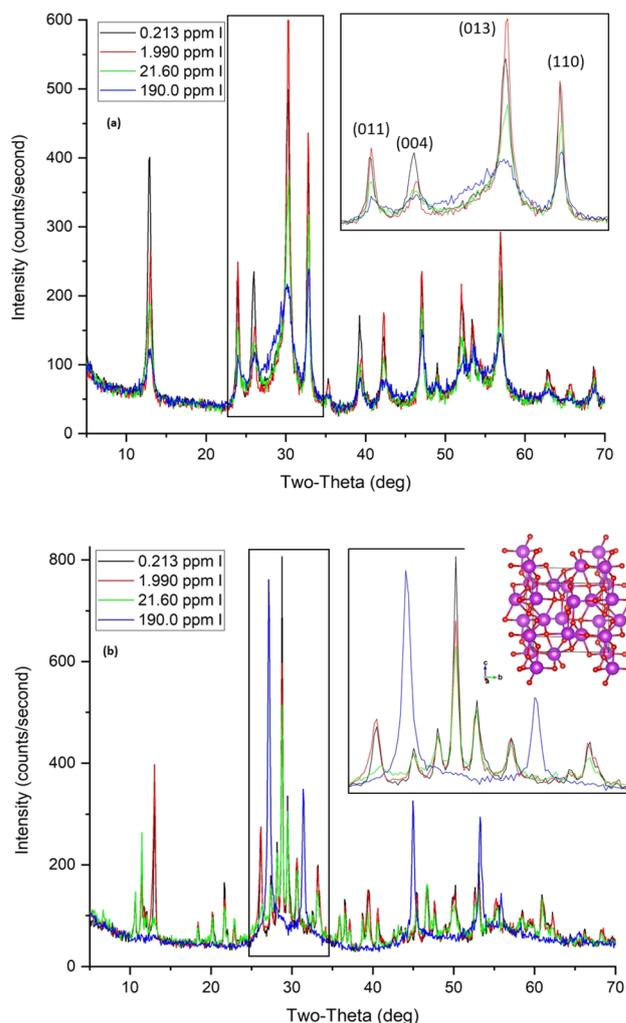
Fig. 12 XRD patterns for BOH (a) and BSN (b) after exposure to different concentrations of iodine for 24 hours, including the crystal structure for  $\delta\text{-Bi}_2\text{O}_3$ . Bi atoms are purple with polyhedral faces shown, O atoms red.
