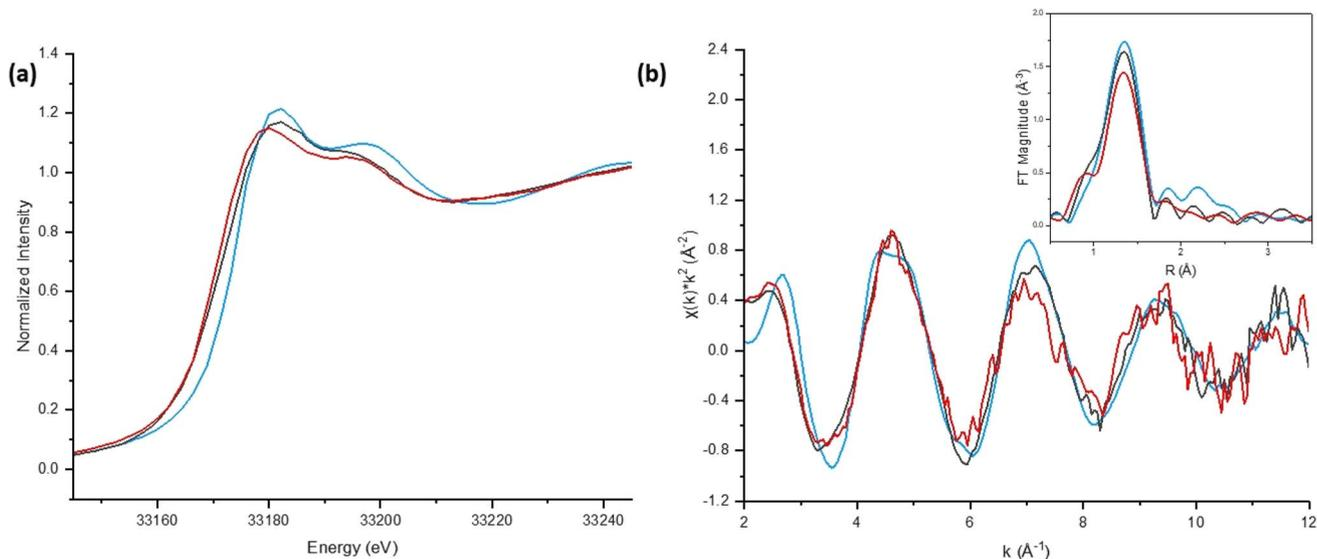
Fig. 13 (a) I K-edge XANES spectra; (b)  $k^2$ -weighted  $\chi(k)$  spectra and Fourier transform magnitude for I (2540 ppm or 0.02 M; sample S) associated with BOH (black line), BSN (red line), and for  $\text{KIO}_3$  (blue line).
