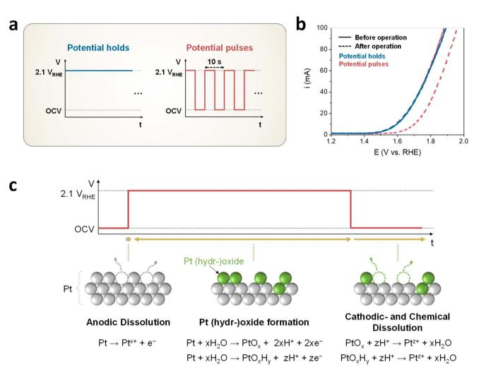
Fig. 2 Potential pulses-induced PTL degradation (a) schematic representation of the potential holds\* and pulses tested in this work. (b) LSV curves for PTLs before and after 50 hours operation of potential holds and potential pulses. (c) Schematic illustration of the Pt coating degradation during the potential pulses. \*potential holds: application of a constant anodic potential.
