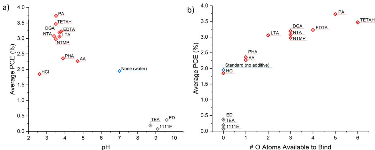
Fig. 8 (a) pH of additives in Table 1 vs. average cell performance of Sb<sub>2</sub>S<sub>3</sub> solar cells made using that additive, (b) number of O atoms available in each additive to bind to Sb<sup>3+</sup> vs. average Sb<sub>2</sub>S<sub>3</sub> solar cell performance. O atoms are considered ‘available to bind’ if they are readily deprotonated to give O<sup>–</sup>, therefore –COOH would count as one available O atom.
