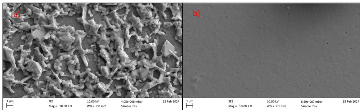
Fig. 2  $\text{Sb}_2\text{S}_3$  film quality shown through SEM images of  $\text{Sb}_2\text{S}_3$  films using (a) no additive and (b) EDTA.
