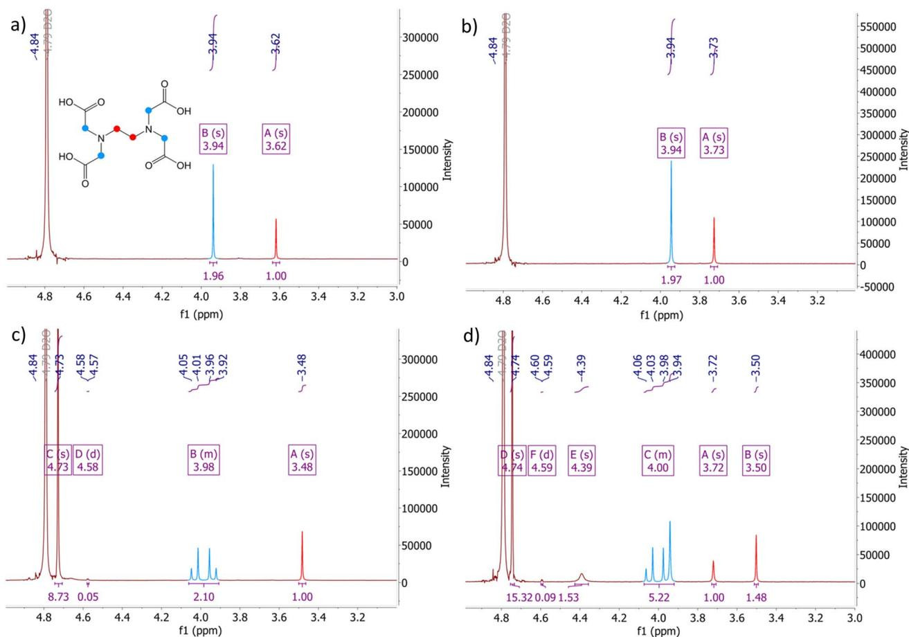
Fig. 3  $^1\text{H}$  NMR spectra of solution containing (a) EDTA in  $\text{D}_2\text{O}$ , showing relative assignments of peaks to groups in EDTA structure, (b) EDTA + STS in  $\text{D}_2\text{O}$ , (c) EDTA + PAT in  $\text{D}_2\text{O}$  and (d) EDTA + STS + PAT in  $\text{D}_2\text{O}$ .
