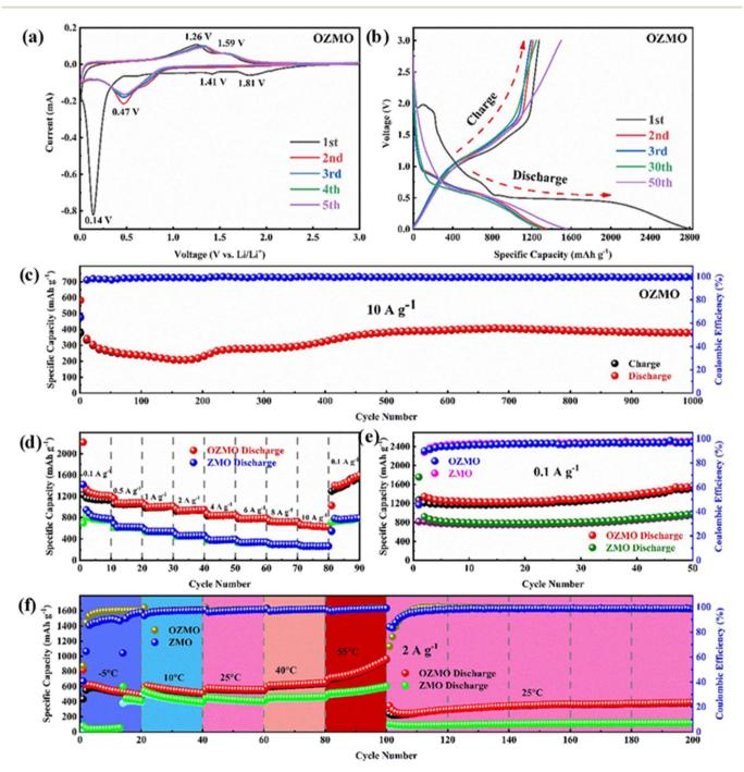
Fig. 10 (a) CV of OZMO at a scan rate of 0.2 mV s<sup>-1</sup>; (b) GCD profile of the OZMO electrodes at 0.1 A g<sup>-1</sup>; (c) cycling stability of OZMO at 10 A g<sup>-1</sup>; (d) rate performance of the OZMO and ZMO electrodes at 0.1–10 A g<sup>-1</sup>; (e) cycling stability of the OZMO and ZMO electrodes at 0.1 A g<sup>-1</sup>; (f) high/low-temperature performance at 2 A g<sup>-1</sup>. Reproduced from ref. 105 with permission from Elsevier, copyright 2021.
