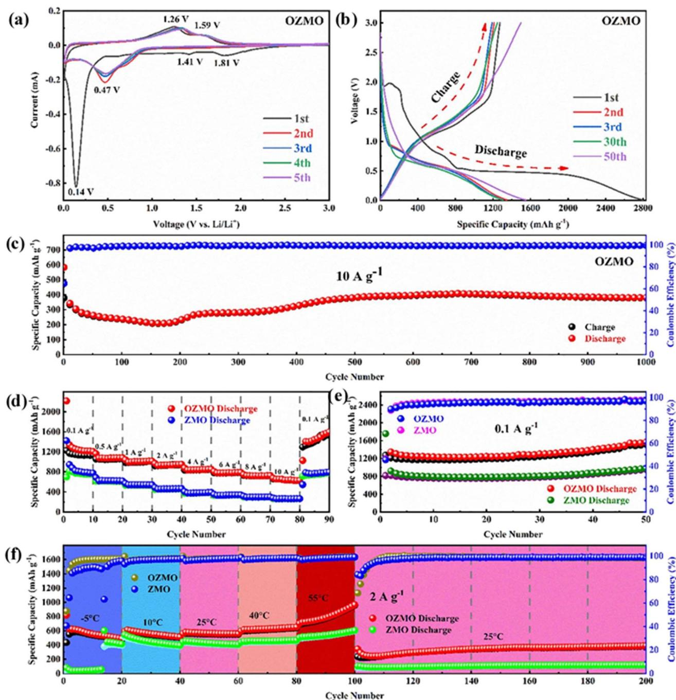
Fig. 10 (a) CV of OZMO at a scan rate of  $0.2 \text{ mV s}^{-1}$ ; (b) GCD profile of the OZMO electrodes at  $0.1 \text{ A g}^{-1}$ ; (c) cycling stability of OZMO at  $10 \text{ A g}^{-1}$ ; (d) rate performance of the OZMO and ZMO electrodes at  $0.1$ – $10 \text{ A g}^{-1}$ ; (e) cycling stability of the OZMO and ZMO electrodes at  $0.1 \text{ A g}^{-1}$ ; (f) high/low-temperature performance at  $2 \text{ A g}^{-1}$ . Reproduced from ref. 105 with permission from Elsevier, copyright 2021.
