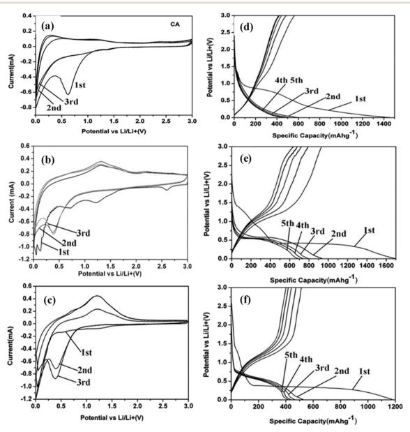
Fig. 9 CV curves of the first three cycles for (a) CA, (b) the 50% ZMO/CA hybrid, and (c) pure ZMO samples at a scan rate of  $0.1 \text{ mV s}^{-1}$  in the voltage range of 0.01-3.0 V. Initial charge-discharge curves of (d) CA, (e) the 50% ZMO/CA hybrid, and (f) pure ZMO samples at a current density of 100 mA g<sup>-1</sup>. Reproduced from ref. 98 with permission from Wiley Online Library, copyright 2014.
