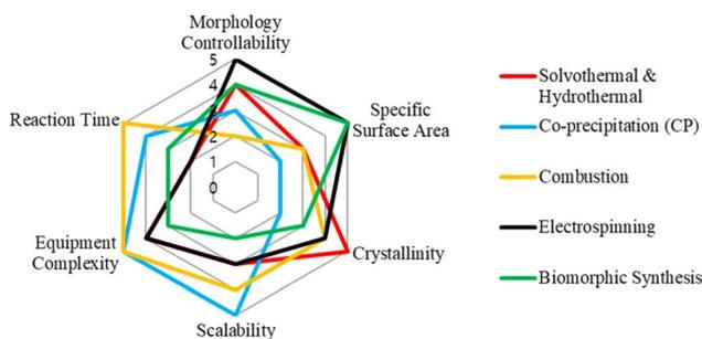
Fig. 5 Polygon radar chart comparing various synthesis methods based on key parameters, including morphology controllability, specific surface area, crystallinity, equipment complexity, and reaction time, which are extracted and explained in Table 3.
