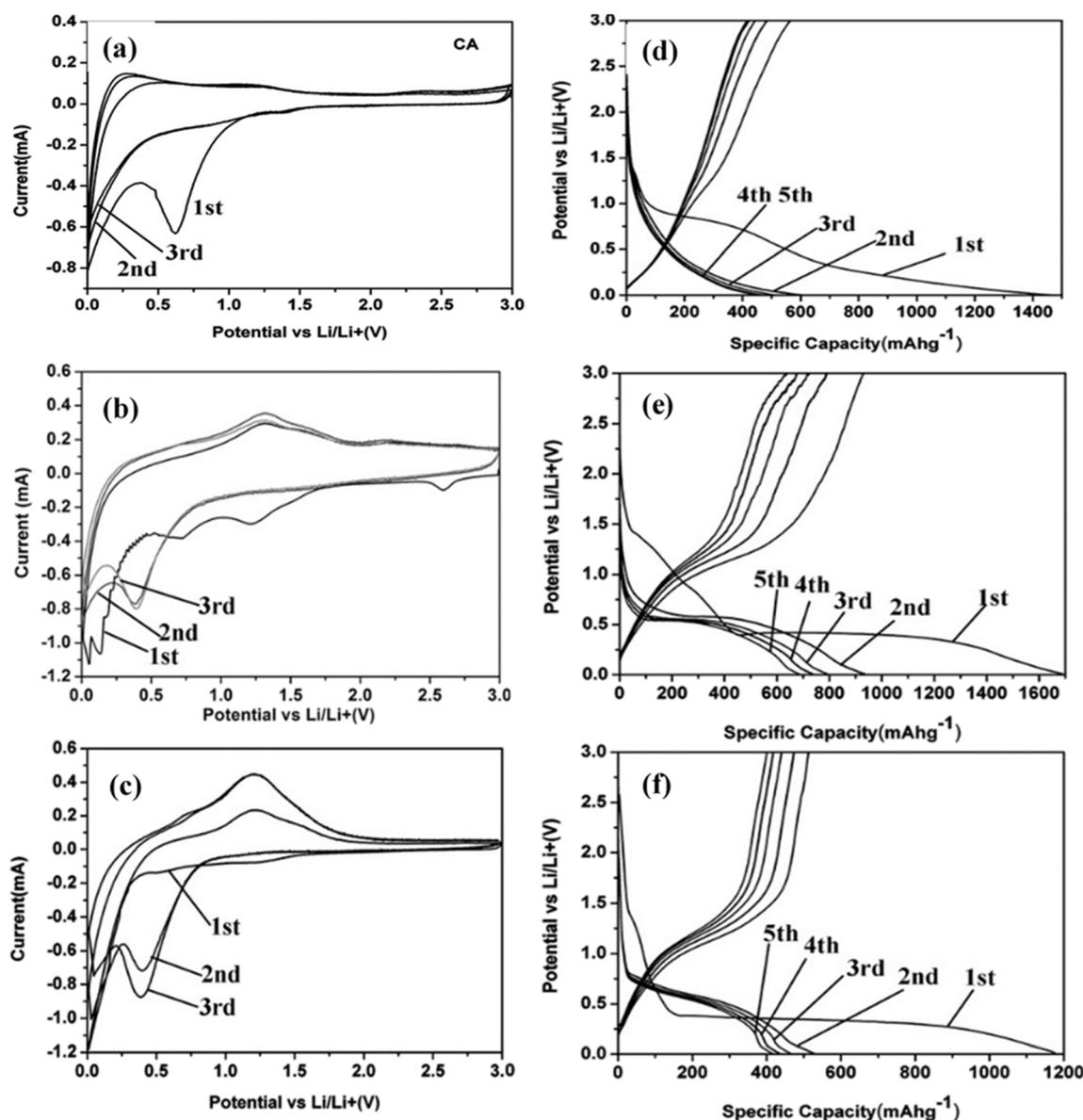
Fig. 9 CV curves of the first three cycles for (a) CA, (b) the 50% ZMO/CA hybrid, and (c) pure ZMO samples at a scan rate of 0.1 mV s<sup>-1</sup> in the voltage range of 0.01–3.0 V. Initial charge–discharge curves of (d) CA, (e) the 50% ZMO/CA hybrid, and (f) pure ZMO samples at a current density of 100 mA g<sup>-1</sup>. Reproduced from ref. 98 with permission from Wiley Online Library, copyright 2014.
