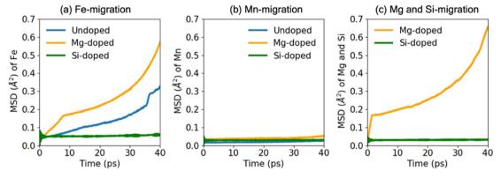
Fig. 4 Mean square displacements (MSD) from AIMD simulations for the out-of-plane migration of (a) Fe, (b) Mn, (c) Mg and Si in undoped  $(Na_xFe_{0.5}Mn_{0.5}O_2)$ , Mg-doped  $(Na_xMg_{0.11}Fe_{0.22}Mn_{0.67}O_2)$  and Si-doped  $(Na_xSi_{0.11}Fe_{0.22}Mn_{0.67}O_2)$ , at the top of charge (x=0.0).
