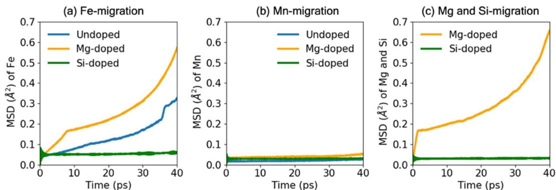
Fig. 4 Mean square displacements (MSD) from AIMD simulations for the out-of-plane migration of (a) Fe, (b) Mn, (c) Mg and Si in undoped ( $\text{Na}_x\text{Fe}_{0.5}\text{Mn}_{0.5}\text{O}_2$ ), Mg-doped ( $\text{Na}_x\text{Mg}_{0.11}\text{Fe}_{0.22}\text{Mn}_{0.67}\text{O}_2$ ) and Si-doped ( $\text{Na}_x\text{Si}_{0.11}\text{Fe}_{0.22}\text{Mn}_{0.67}\text{O}_2$ ), at the top of charge ( $x = 0.0$ ).
