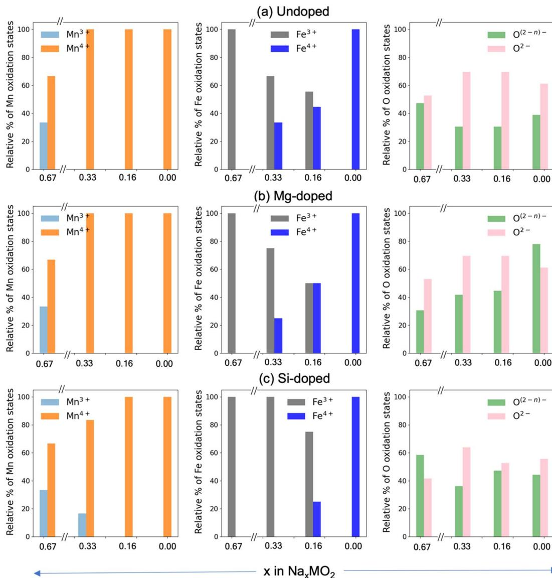
Fig. 2 Redox-active ions in (a) undoped  $\text{Na}_x\text{Fe}_{0.5}\text{Mn}_{0.5}\text{O}_2$ , (b) Mg-doped  $\text{Na}_x\text{Mg}_{0.11}\text{Fe}_{0.22}\text{Mn}_{0.67}\text{O}_2$ , and (c) Si-doped  $\text{Na}_x\text{Si}_{0.11}\text{Fe}_{0.22}\text{Mn}_{0.67}\text{O}_2$  showing the relative % amount of the different oxidation states of Mn, Fe and O as a function of Na content ( $x$ ) from the pristine material to high charge states ( $x = 0.33, 0.16, 0.00$ ).
