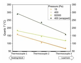
Fig. 3 T gradient across the cold zone of the quartz tube under different  $p_T$ . The positions of the thermocouples are illustrated in Fig. 2b. In one case, part of the cold zone was wrapped in insulation tape. Data points for 15 and 400 Pa nearly overlap.
