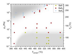
Fig. 6 Experimental  $p_S$ -T phase diagram for the Ba-S system. Following the sulfurization of BaS<sub>2</sub> precursors, the graph indicates whether some BaS or BaS<sub>3</sub> formed or if no phase transformation occurred. The shaded areas indicate the estimated regions of stability for the different phases. The measured  $T_S$  was mapped to a  $p_S$ equivalent assuming that saturation was reached.
