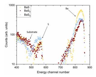
Fig. 5 Raw data from RBS measurements. Yellow dots, red squares, and blue stars represent representative samples in which either BaS, BaS<sub>2</sub>, or BaS<sub>3</sub> is the predominant phase, respectively. The peaks around energy channels 560 and 840 correspond to S and Ba, respectively. Counts below energy channel 500 originate from the substrate.
