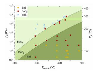
Fig. 7 Predicted  $p_S-T$  phase diagram for the Ba-S system. Colored regions indicate which material is most stable at a given  $T_{\text{sample}}$  and  $p_{\text{S}}$ . The overlapped scatter points correspond to experimental data. The measured  $T_S$  was mapped to a  $p_S$  equivalent, assuming that saturation was reached
