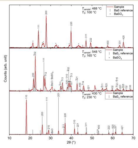
Fig. 4 GI-XRD patterns of representative samples in which either BaS, BaS<sub>2</sub>, or BaS<sub>3</sub> predominates, together with their relative reference patterns.<sup>21–23</sup> Peaks belonging to BaSO<sub>3</sub> or BaSO<sub>4</sub> impurities are marked with an asterisk.<sup>24,25</sup>
