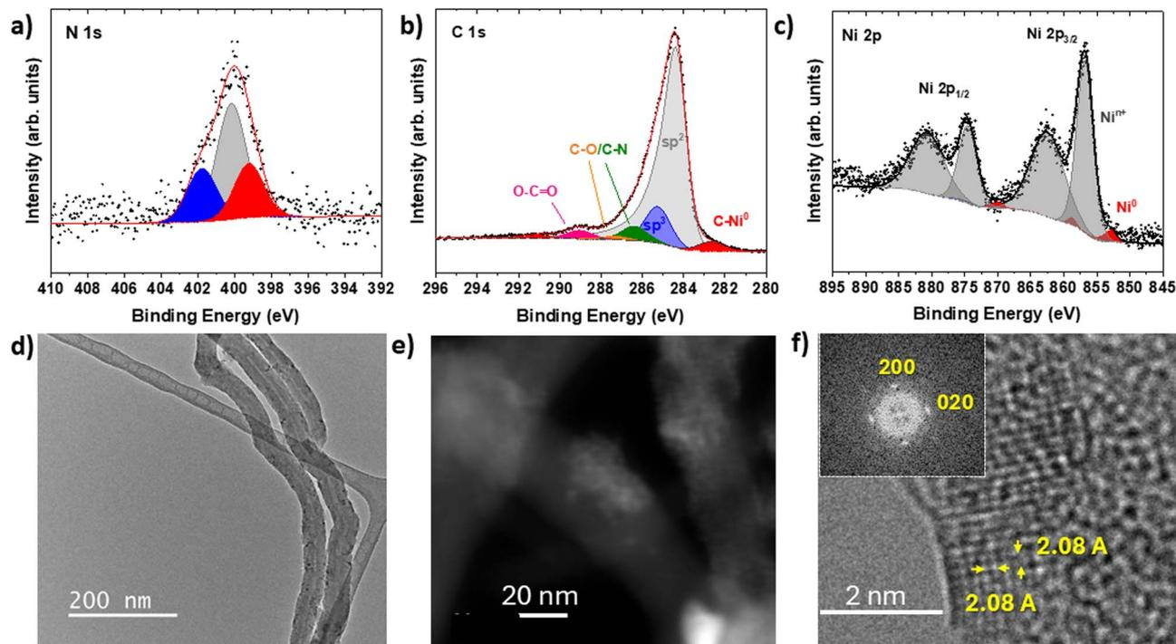
Fig. 1 (a) XPS narrow scans of N 1s, (b) C 1s, (c) Ni 2p and (d) TEM image of **10**, (e) HAADF-STEM image of **10** and (f) HRTEM-atomic resolved image of NiNCs of **10** with the corresponding lattice fringes (inset: FFT).
