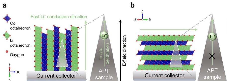
Fig. 1 Schematics illustrating the effect of crystallographic orientation on *in situ* delithiation in APT analysis for LTMOs. (a) When fast Li-ion conducting directions are parallel to the applied field, severe *in situ* delithiation occurs due to Li<sup>+</sup> migration along high mobility directions. (b) When the Li-ion blocking direction is parallel to the applied field, Li<sup>+</sup> motion and *in situ* delithiation is suppressed.
