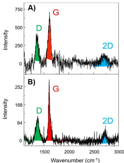
Fig. 7 Raman spectra of the anode surfaces retrieved from (A) the cell subjected to ESC conditions and (B) pristine cell discharged to 0 V.
