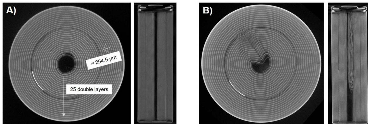
Fig. 1 CT images showing the cross-sectional and longitudinal views of a commercial 21700 cell (A) pristine cell discharged to 0 V and (B) cell subjected to ESC conditions.
