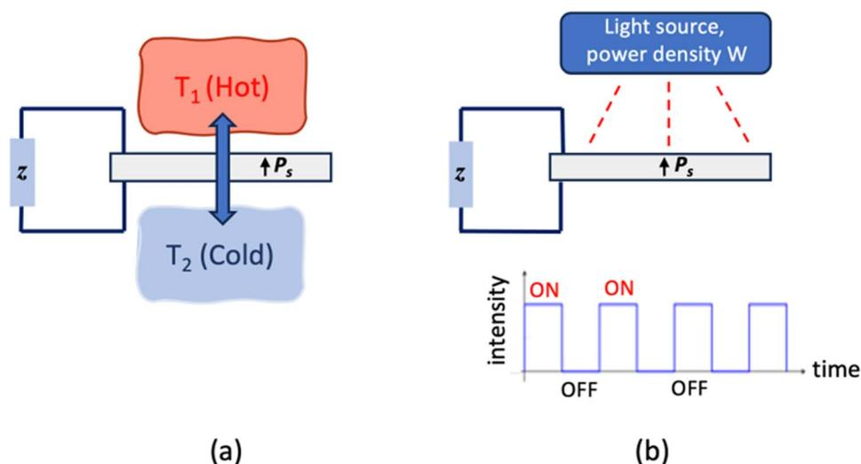
Fig. 2 (a) Cycling between two temperatures,  $T_1$  and  $T_2$ , (b) modulated heat source, leading to temperature fluctuations where the final temperature of the pyroelectric material depends on the heat capacity of the material.
