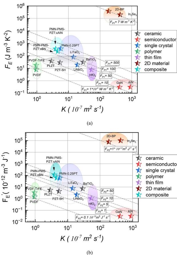
Fig. 3 Ashby charts. (a) Selection of materials with high  $F_{P1} = F_E K$ , lines of constant  $F_{P1}$  can be drawn via a gradient of  $n = -1$ , based on eqn (26). (b) Selection of materials with high  $F_{P2} = F'_E K = F_{P1}/\epsilon_E^2$ , lines of constant  $F_{P2}$  can be drawn via a gradient of  $n = -1$ , based on eqn (27).
