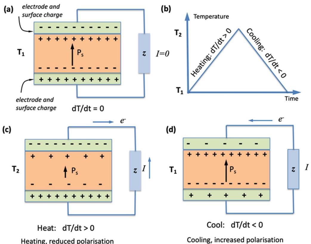
Fig. 1 Schematic of the pyroelectric effect (a) initial state,  $dT/dt = 0$ , where current  $I = 0$ , (b) heating profile, (c) heating cycle ( $dT/dt > 0$ ) leads to a decrease in polarisation and current flow, (d) cooling cycle ( $dT/dt < 0$ ) leads to an increase in polarisation and current flow in opposite direction.
