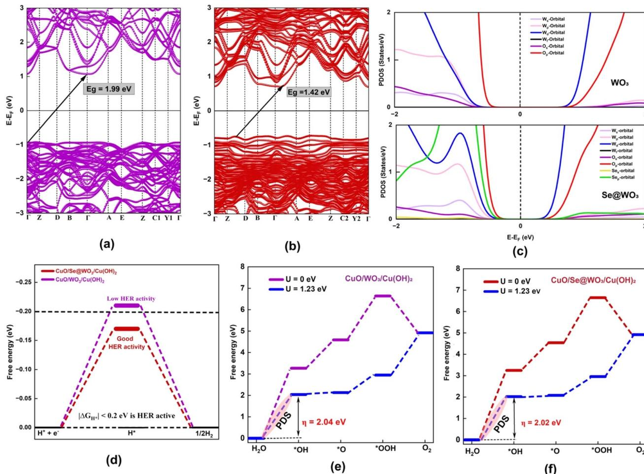
Fig. 4 Electronic band structures of (a)  $\text{WO}_3$ , (b)  $\text{Se@WO}_3$ , and (c) projected density of states (PDOS) plots of  $\text{WO}_3$  and  $\text{Se@WO}_3$ . Free energy profile for the (d) HER and (e) and (f) OER in  $\text{CuO/WO}_3/\text{Cu(OH)}_2$  and  $\text{CuO/Se@WO}_3/\text{Cu(OH)}_2$ .
