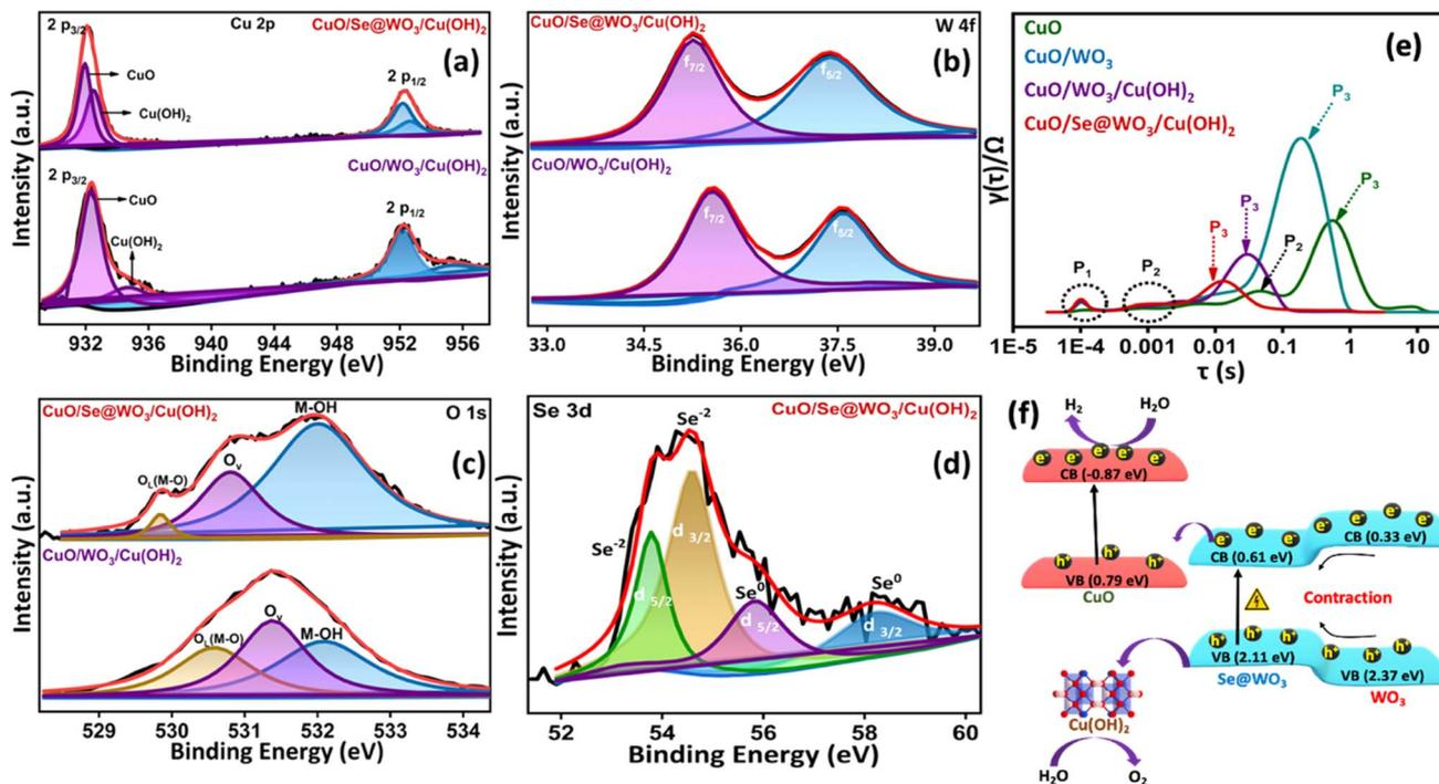
Fig. 3 High-resolution XPS spectra of (a) Cu 2p, (b) W 4f and (c) O 1s for CuO/WO<sub>3</sub>/Cu(OH)<sub>2</sub> (bottom) and CuO/Se@WO<sub>3</sub>/Cu(OH)<sub>2</sub> (top); (d) XPS core level spectra for Se 3d for CuO/Se@WO<sub>3</sub>/Cu(OH)<sub>2</sub>; (e) DRT analysis performed from EIS data; (f) schematic representing the electron transfer process across the heterojunction for overall water splitting.
