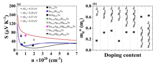
Fig. 6 (a) Pisarenko plot showing the Seebeck coefficient *versus* carrier concentration for SnTe, considering contributions from both light and heavy hole valence bands with varying energy gaps ( $\Delta E \approx 0.35$  eV, 0.28 eV, 0.27 eV and 0.10 eV).<sup>47</sup> (b) Density of states effective mass for pristine and doped SnTe samples. Ag, Mg, and Bi doping increase the effective mass, with Mg doping alone showing a significant increase.
