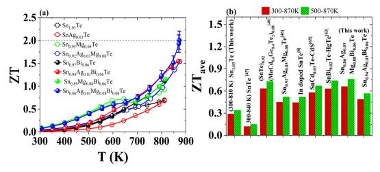
Fig. 8 Thermoelectric performance comparison of doped SnTe compounds: (a) ZT values as a function of temperature for various doped SnTe variants, <sup>65</sup> and (b) average ZT values over different temperature ranges compared with other reported materials.
