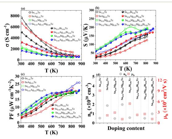
Fig. 5 Temperature-dependent thermoelectric properties of polycrystalline and doped SnTe samples. (a) Electrical conductivity (σ). (b) Seebeck coefficient (S). (c) Power factor (PF). (d) Carrier concentration  $(n_{\rm h})$  and mobility  $(\mu_{\rm h})$  vary with doping
