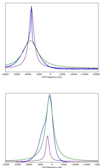
Fig. 6 Solid state, wideline  $^{31}\text{P}$  (top) and  $^{11}\text{B}$  (bottom) NMR spectrum of  $[\text{P}_{4444}][\text{B}(\text{bdo})_2]$  at 253 K ( $-20$  °C) showing deconvolution into the broad (static) contribution in green and sharper (mobile) contributions in purple.
