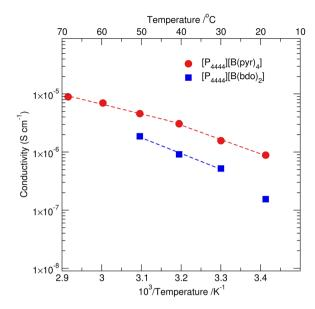
Fig. 4 Arrhenius plot of the conductivity of  $[P_{4444}][B(pyr)_4]$  (red) and  $[P_{4444}][B(bdo)_2]$  (blue). Dashed lines represent fits to the Arrhenius equation with activation energy,  $E_a$ , of 51.9 kJ mol<sup>-1</sup> for  $[P_{4444}][B(bdo)_2]$  between 303–323 K, 32.2 kJ mol<sup>-1</sup> for  $[P_{4444}][B(pyr)_4]$  between 312–343 K and 47.4 kJ mol<sup>-1</sup> for  $[P_{4444}][B(pyr)_4]$  between 293–313 K (all with  $r^2 > 0.996$ ).
