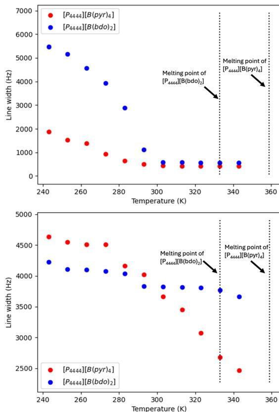
Fig. 7 Line width (Hz) of <sup>31</sup>P (top) and <sup>11</sup>B (bottom) static NMR signals from [P<sub>4444</sub>][B(bdo)<sub>2</sub>] and [P<sub>4444</sub>][B(pyr)<sub>4</sub>] over the temperature range 243–343 K.
