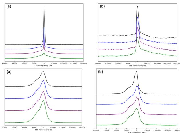
Fig. 5 Stacked wide line static solid state  $^{31}\text{P}$  (top) and  $^{11}\text{B}$  (bottom) NMR signals from at various temperatures  $[\text{P}_{4444}][\text{B}(\text{bdo})_2]$  (a, left) and  $[\text{P}_{4444}][\text{B}(\text{pyr})_4]$  (b, right) at  $T = 243$  K (green), 273 K (purple), 303 K (blue), and 343 K (black).
