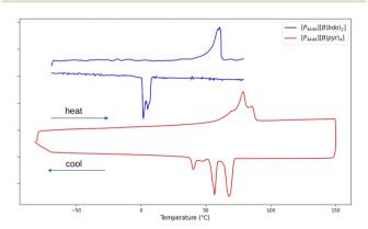
Fig. 3 DSC scan of  $[P_{4444}][B(pyr)_4]$  (red) and  $[P_{4444}][B(bdo)_2]$  (blue) with a scan rate of 10 °C min<sup>-1</sup> (endothermic up).
