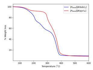
Fig. 2 TGA profiles from 50-600 °C of  $[P_{4444}][B(pyr)_4]$  (red) and [P<sub>4444</sub>][B(bdo)<sub>2</sub>] (blue).
