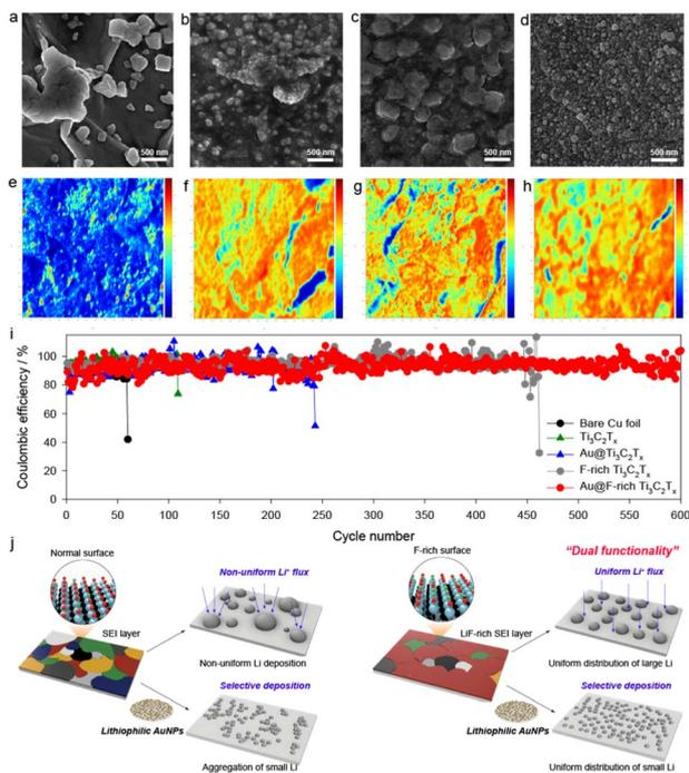
Fig. 4 Li deposition behavior and cyclic performance of MXene. SEM and SIMS images of (a) and (e) Ti<sub>3</sub>C<sub>2</sub>T<sub>x</sub>, (b) and (f) Au@Ti<sub>3</sub>C<sub>2</sub>T<sub>x</sub>, (c) and (g) F-rich Ti<sub>3</sub>C<sub>2</sub>T<sub>x</sub>, (d) and (h) Au@F-rich Ti<sub>3</sub>C<sub>2</sub>T<sub>x</sub> and (e) Ti<sub>3</sub>C<sub>2</sub>T<sub>x</sub>. (i) Cycle life of MXene at 1.0 mA cm<sup>-2</sup>@1.0 mA h cm<sup>-2</sup>. (j) Schematic illustration of Li deposition on MXene.
