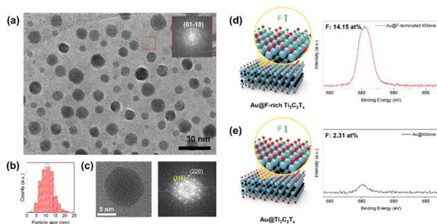
Fig. 2 Identification of the synthesized Au NPs on F-rich  $\text{Ti}_3\text{C}_2\text{T}_x$  MXene and fluorine terminations. (a) TEM image of Au@F-rich  $\text{Ti}_3\text{C}_2\text{T}_x$  MXene, (b) particle size distribution of Au NPs, (c) high resolution TEM (HRTEM) bright field image of Au NP and the corresponding FFT pattern. F 1s XPS spectra of (d) Au@F-rich  $\text{Ti}_3\text{C}_2\text{T}_x$  and (e) as prepared Au@ $\text{Ti}_3\text{C}_2\text{T}_x$  (before Li deposition).
