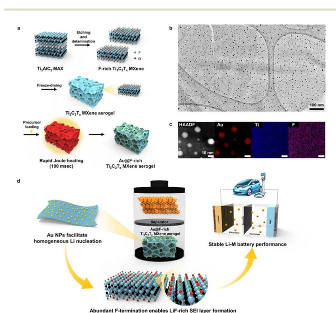
**Fig. 1** Synthesis of Au NPs on surface termination controlled  $\text{Ti}_3\text{C}_2\text{T}_x$  MXene by rapid Joule heating for Li-metal battery anodes. (a) Chemical wet etching and rapid Joule heating synthesis of Au@F-rich  $\text{Ti}_3\text{C}_2\text{T}_x$  MXene. (b) TEM image and (c) TEM-EDS image of Au@F-rich  $\text{Ti}_3\text{C}_2\text{T}_x$  MXene. (d) Schematic illustration of Au@F-rich  $\text{Ti}_3\text{C}_2\text{T}_x$  MXene as a Li-metal battery anode.
