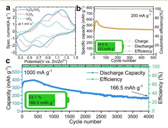
Fig. 6 CV curves of  $V_2O_5$ ,  $VO_2$ , and  $V_2O_5/VO_2$  photocathode-based ZIBs at a scan rate of 1 mV s<sup>-1</sup> in light (a) and the cycling performances of  $V_2O_5/VO_2$  photocathode-based ZIBs conducted at current densities of 200 mA  $g^{-1}$  (b) and 1000 mA  $g^{-1}$  (c) of the  $V_2O_5/VO_2$  photocathodebased ZIBs in the light condition.
