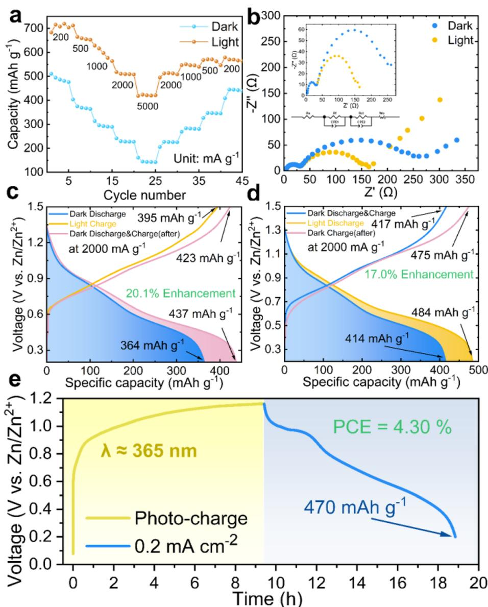
Fig. 5 Rate performances (a), EIS spectra (b), light charge and dark discharge curves obtained at a current density of 2000 mA g<sup>-1</sup> (c), dark charge and light discharge curves obtained at 2000 mA g<sup>-1</sup> using a full-spectrum Xe lamp (d), and the light charge and dark discharge curve obtained using a single-wavelength LED light of ~365 nm of the as-fabricated photo-ZIBs (e).
