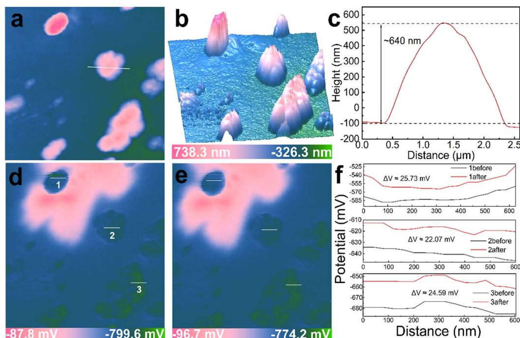
Fig. 3 Two-dimensional (a) and three-dimensional (b) KPFM images, actual height distribution map of the white line section (c), the corresponding KPFM surface potential images without (d) and with (e) light irradiation, and the comparisons of surface potentials with/without light irradiation of the as-prepared  $V_2O_5/VO_2$  nanospheres (f).
