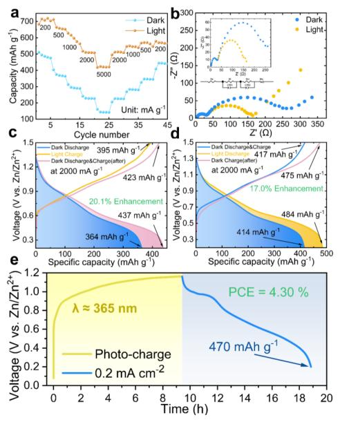
Fig. 5 Rate performances (a), EIS spectra (b), light charge and dark discharge curves obtained at a current density of 2000 mA g $^{-1}$  (c), dark charge and light discharge curves obtained at 2000 mA g $^{-1}$  using a full-spectrum Xe lamp (d), and the light charge and dark discharge curve obtained using a single-wavelength LED light of  $\sim$ 365 nm of the as-fabricated photo-ZIBs (e).
