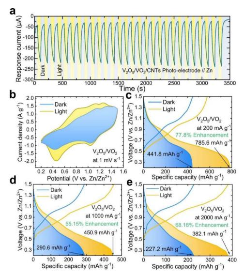
Fig. 4 Photocurrent response (a), CV curves obtained within a potential window of 0.2–1.5 V under dark and light conditions (b), chargedischarge curves obtained at current densities of 200 mA  $\rm g^{-1}$  (c), 1000 mA  $\rm g^{-1}$  (d), and 2000 mA  $\rm g^{-1}$  (e) under dark and light conditions of the asfabricated ZIBs cells employing  $\rm V_2O_5/VO_2$  as photocathodes.
