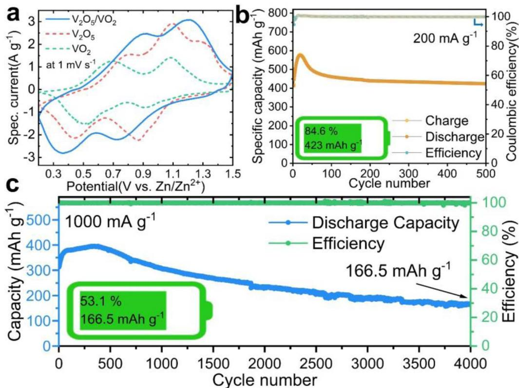
Fig. 6 CV curves of  $\text{V}_2\text{O}_5$ ,  $\text{VO}_2$ , and  $\text{V}_2\text{O}_5/\text{VO}_2$  photocathode-based ZIBs at a scan rate of  $1 \text{ mV s}^{-1}$  in light (a) and the cycling performances of  $\text{V}_2\text{O}_5/\text{VO}_2$  photocathode-based ZIBs conducted at current densities of  $200 \text{ mA g}^{-1}$  (b) and  $1000 \text{ mA g}^{-1}$  (c) of the  $\text{V}_2\text{O}_5/\text{VO}_2$  photocathode-based ZIBs in the light condition.
