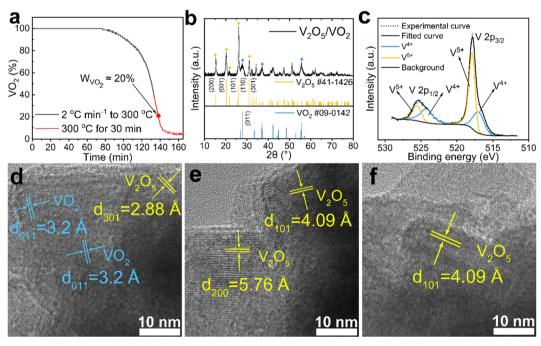
Fig. 2 TGA curve (a), XRD pattern (b), XPS spectra (c), and HR-TEM images (d-f) of the V<sub>2</sub>O<sub>5</sub>/VO<sub>2</sub> hollow nanospheres.
