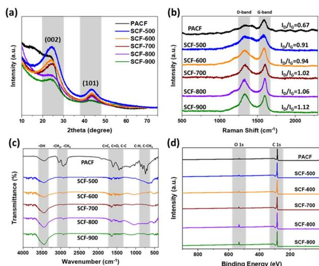
Fig. 3 (a) XRD patterns, (b) Raman spectra, (c) FT-IR spectra, and (d) XPS survey scan of the PACF and SCF samples.
