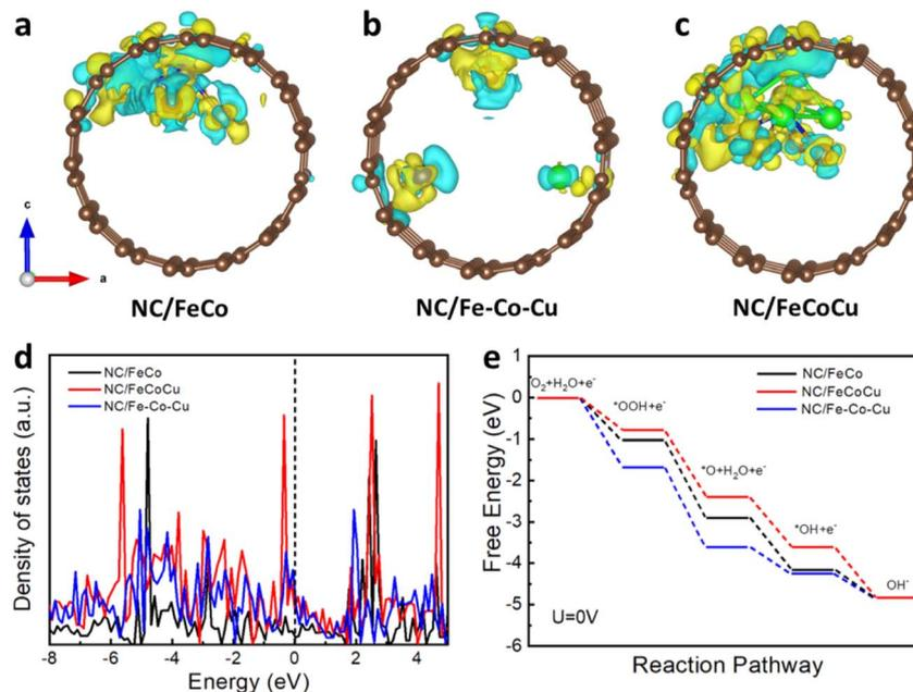
Fig. 5 The optimized geometry models of (a) N-doped carbon/FeCo, (b) N-doped carbon/Fe-Co-Cu, and (c) N-doped carbon/FeCoCu. Yellow regions indicate an increase in charge density and blue regions represent a decrease in charge density. (d) The projected density of states and (e) free-energy landscape of intermediates in the standard four electron transfer reaction pathway for ORR catalysis by the three electrocatalysts.
