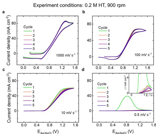
Fig. 1 Series of CVs of GC RDE in 0.2 M HT/0.5 M NaCl solution collected at 900 rpm for the following scan rates: (a) 1000 mV s<sup>-1</sup>, (b) 100 mV s<sup>-1</sup>, (c) 10 mV s<sup>-1</sup>, and (d) 0.5 mV s<sup>-1</sup>.
