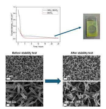
Fig. 3 Top: chronoamperometry stability testing of BiVO<sub>4</sub> and WO<sub>3</sub>-|BiVO<sub>4</sub> electrodes at 1.23  $V_{\rm RHE}$  in 0.1 M KPi (pH 7) and photograph showing degradation of the irradiated area of the WO<sub>3</sub>|BiVO<sub>4</sub> electrode after the 24 hours test. Below: SEM images of WO<sub>3</sub>|BiVO<sub>4</sub> before and after the stability test. PEC measurements were taken under simulated sunlight (AM 1.5 G, 1 sun).
