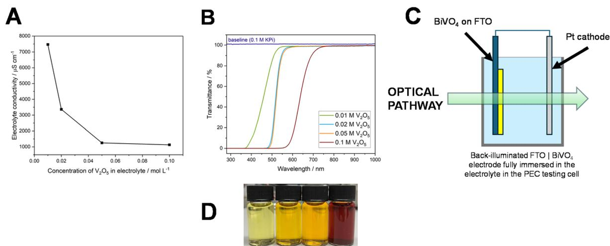
Fig. 4 Conductivity (A) and UV-Vis transmittance (B) of 0.1 M KPi electrolyte (pH 7) with various concentrations of  $\text{V}_2\text{O}_5$ . Optical pathway of the photoelectrochemical cell used for preliminary PEC testing of  $\text{WO}_3|\text{BiVO}_4$  electrodes (C). Photograph of 0.1 M KPi electrolyte containing  $\text{V}_2\text{O}_5$  electrolyte with concentrations of 0.01 M, 0.02 M, 0.05 M and 0.1 M from left to right (D).
