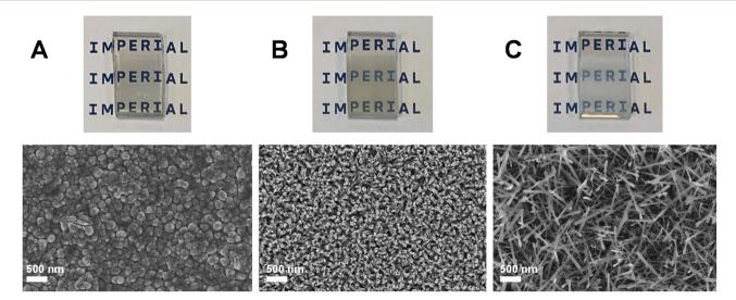
Fig. 6 SEM images of WO<sub>3</sub> synthesised at different AA-CVD reaction temperatures. Planar WO<sub>3</sub> synthesised at 325 °C (A), hybrid WO<sub>3</sub> synthesised at 350 °C (B), nanoneedle WO<sub>3</sub> synthesised at 375 °C (C). Accompanying photographs shown in A, B and C insets.
