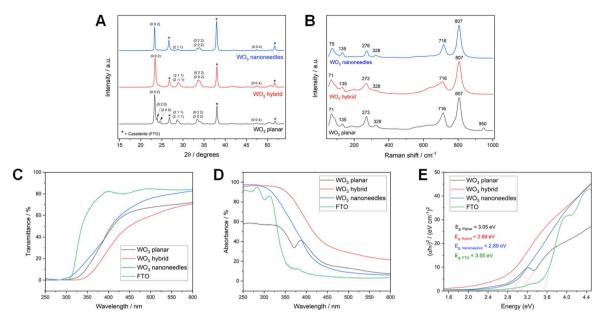
Fig. 7 XRD patterns (A) and Raman spectra (B), UV-Vis transmittance (C), UV-Vis absorbance (D) and Tauc plots (E) of WO<sub>3</sub> with planar, hybrid and nanoneedle morphologies, deposited on FTO glass
