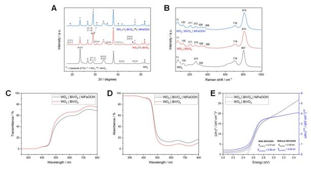
Fig. 11 XRD patterns (A) and Raman spectra (B) of WO<sub>3</sub>, WO<sub>3</sub>|BiVO<sub>4</sub> and WO<sub>3</sub>|BiVO<sub>4</sub>|NiFeOOH photoanodes (all of hybrid WO<sub>3</sub> nanoneedle morphology), deposited on FTO glass. UV-Vis transmittance (C), absorbance (D) and Tauc plots (E) of WO<sub>3</sub>|BiVO<sub>4</sub> with and without NiFeOOH, deposited on FTO glass.
