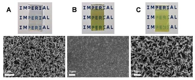
Fig. 2 SEM images and accompanying photographs of the photoanodes used in the initial scoping and validation study.  $WO_3$  nanoneedles on FTO (A),  $BiVO_4$  on FTO (B) and  $BiVO_4$  conformally coated on the  $WO_3$  nanoneedles to form a  $WO_3$   $BiVO_4$  heterojunction (C).
