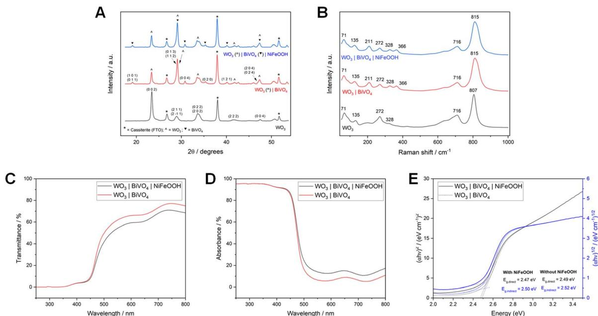
Fig. 11 XRD patterns (A) and Raman spectra (B) of  $\text{WO}_3$ ,  $\text{WO}_3|\text{BiVO}_4$  and  $\text{WO}_3|\text{BiVO}_4|\text{NiFeOOH}$  photoanodes (all of hybrid  $\text{WO}_3$  nanoneedle morphology), deposited on FTO glass. UV-Vis transmittance (C), absorbance (D) and Tauc plots (E) of  $\text{WO}_3|\text{BiVO}_4$  with and without  $\text{NiFeOOH}$ , deposited on FTO glass.
