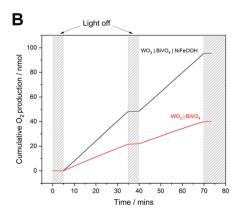
Fig. 14 Normalised oxygen production rate with and without NiFeOOH co-catalyst (A) and cumulative oxygen production over time (B) under white light irradiation (100 mW cm<sup>-2</sup>).
