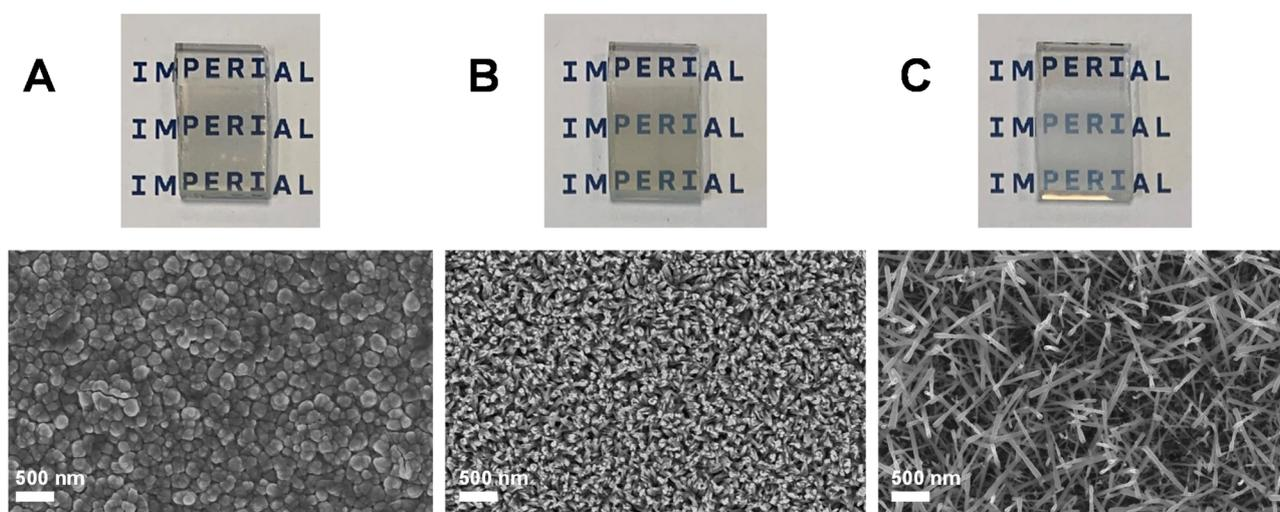
Fig. 6 SEM images of  $\text{WO}_3$  synthesised at different AA-CVD reaction temperatures. Planar  $\text{WO}_3$  synthesised at 325 °C (A), hybrid  $\text{WO}_3$  synthesised at 350 °C (B), nanoneedle  $\text{WO}_3$  synthesised at 375 °C (C). Accompanying photographs shown in A, B and C insets.
