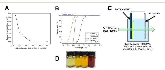
Fig. 4 Conductivity (A) and UV-Vis transmittance (B) of 0.1 M KPi electrolyte (pH 7) with various concentrations of V<sub>2</sub>O<sub>5</sub>. Optical pathway of the photoelectrochemical cell used for preliminary PEC testing of  $WO_3|BiVO_4|$  electrodes (C). Photograph of 0.1 M KPi electrolyte containing  $V_2O_5|$ electrolyte with concentrations of 0.01 M, 0.02 M, 0.05 M and 0.1 M from left to right (D).
