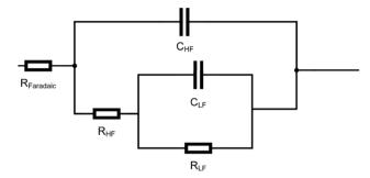
Fig. 1 Equivalent electrical circuit used for fitting PEIS spectra. HF = high frequency, LF = low frequency.
