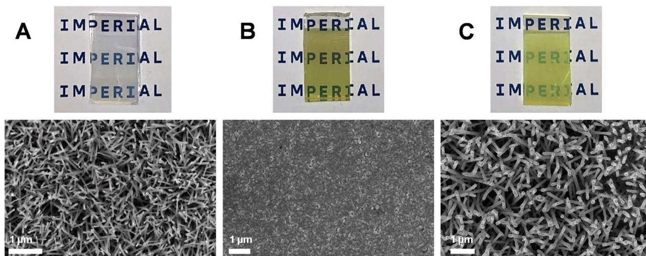
Fig. 2 SEM images and accompanying photographs of the photoanodes used in the initial scoping and validation study.  $\text{WO}_3$  nanoneedles on FTO (A),  $\text{BiVO}_4$  on FTO (B) and  $\text{BiVO}_4$  conformally coated on the  $\text{WO}_3$  nanoneedles to form a  $\text{WO}_3|\text{BiVO}_4$  heterojunction (C).
