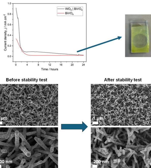
Fig. 3 Top: chronoamperometry stability testing of  $\text{BiVO}_4$  and  $\text{WO}_3|\text{BiVO}_4$  electrodes at  $1.23 V_{\text{RHE}}$  in 0.1 M KPi (pH 7) and photograph showing degradation of the irradiated area of the  $\text{WO}_3|\text{BiVO}_4$  electrode after the 24 hours test. Below: SEM images of  $\text{WO}_3|\text{BiVO}_4$  before and after the stability test. PEC measurements were taken under simulated sunlight (AM 1.5 G, 1 sun).
