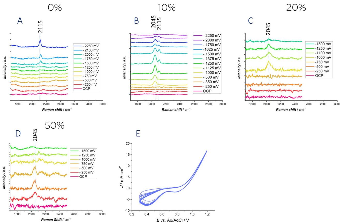
Fig. 6 Potential-dependent *in situ* SERS spectra measured at an ORC-treated polycrystalline Au electrode in contact with the Ethaline DES with the indicated water contents. Panels (A–D) report the spectra recorded in the  $\text{CN}^-$  stretching range for different hydration levels. (E) A typical ORC cycle adopted for the achievement of the SERS effect.
