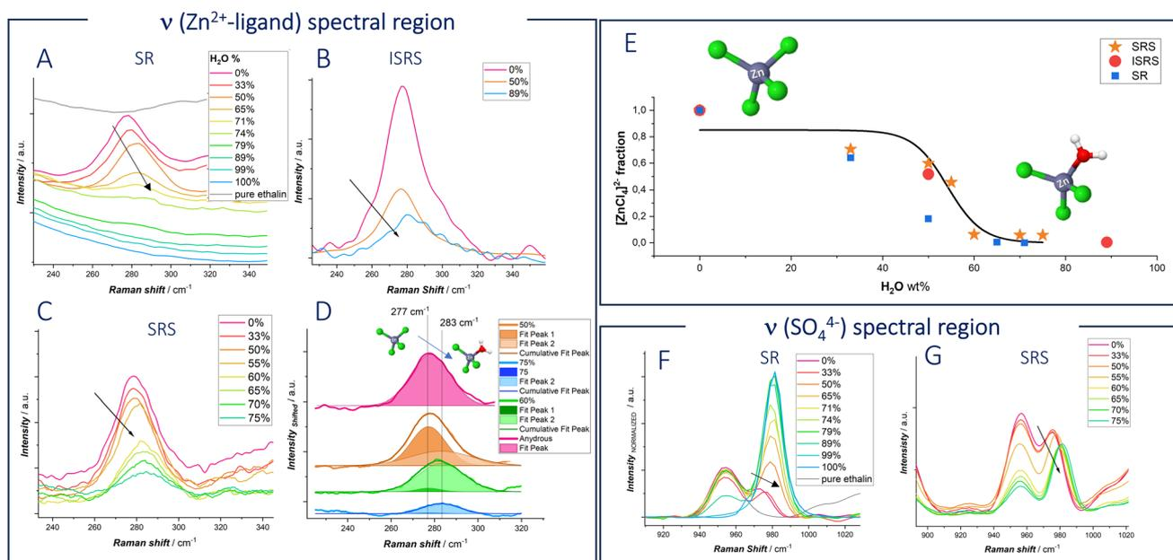
Fig. 4 (A–D)  $\nu(\text{Zn-ligand})$  and (F and G)  $\nu(\text{SO}_4^{2-})$  spectra for pure anhydrous ethaline and DESEG-H<sub>2</sub>O hybrid electrolytes with the indicated water wt%: (A) spontaneous Raman; (B) Impulsive Stimulated Raman Scattering (ISRS); (C) Stimulated Raman Scattering (SRS); (D) fitted SRS curves. (E)  $[\text{ZnCl}_4]^{2-}$  fraction estimated for the fitting of the spectra of panels (A–D). (F) Spontaneous Raman. (G) SRS.
