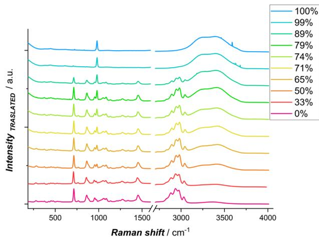
Fig. 3 Spontaneous Raman spectra of DESEG-H<sub>2</sub>O hybrid electrolytes with different wt% (0%, 50%, 65%, 71%, 74%, 79%, 89%, 99% and 100%); the spectra are shifted vertically for clarity.
