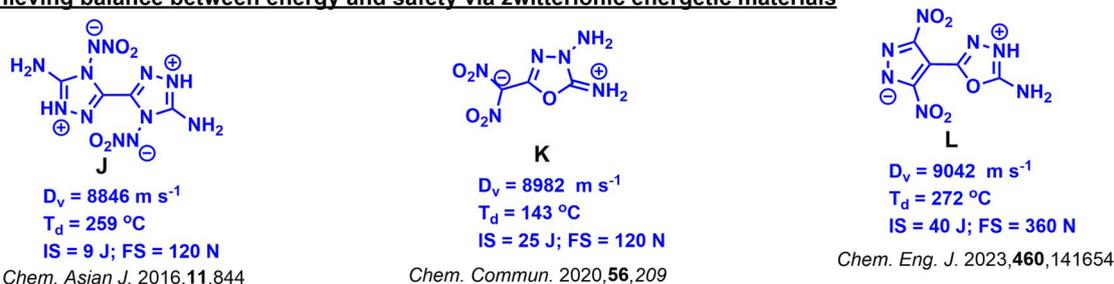
**Scheme 1** (a) Impact of positional isomerism on chemical reactivity and energetic properties of products obtained which highlights the critical role of precursor selection; (b) selected trinitromethyl-triazole and dinitromethyl-triazole functionalization, which showcase significant improvement in detonation velocity, pressure, and density. (c) Selected zwitterionic compounds for improved density, stability, and energetic properties through charge separation.
