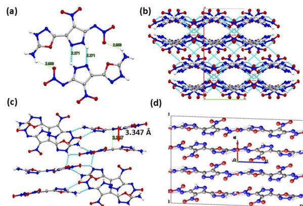
Fig. 2 (a) Hydrogen bonding interactions with a maximum D-D distance of 2.9 Å and a minimum angle of  $120^\circ$ . (b) Zigzag hydrogen bonding network (3.347 Å). (c) Layered packing with  $\pi-\pi$  stacking interactions (3.347 Å). (d) Compact lattice showing tight molecular interlocking along the  $b$ -axis.
