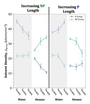
Fig. 5 Comparing the effect on  $\rho_{\rm group}$  of changing the relative atomic length of P and NP groups for hydroxyl Pn:NPn systems. The left half is plotted with increasing length of NP group, while the right is plotted with increasing length of P group. The same sets of three systems are compared under water (grey) and hexane (white). Error bars are a 95% confidence interval across six simulated surfaces.
