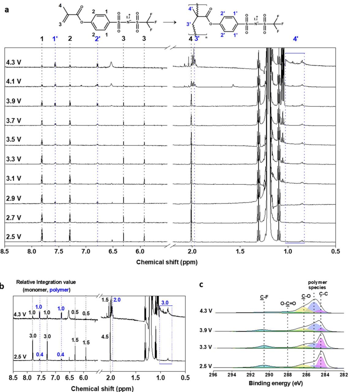
Fig. 5 Consumption pattern of LiMPTFSI in the graphite/NCM cell at different voltages during the first charging process. (a)  $^1\text{H}$  NMR spectra of LiMPTFSI, (b) relative integration values of monomer and polymer at 2.5 and 4.3 V, and (c) C 1s XPS spectra of the graphite anode surface during the initial charge process.
