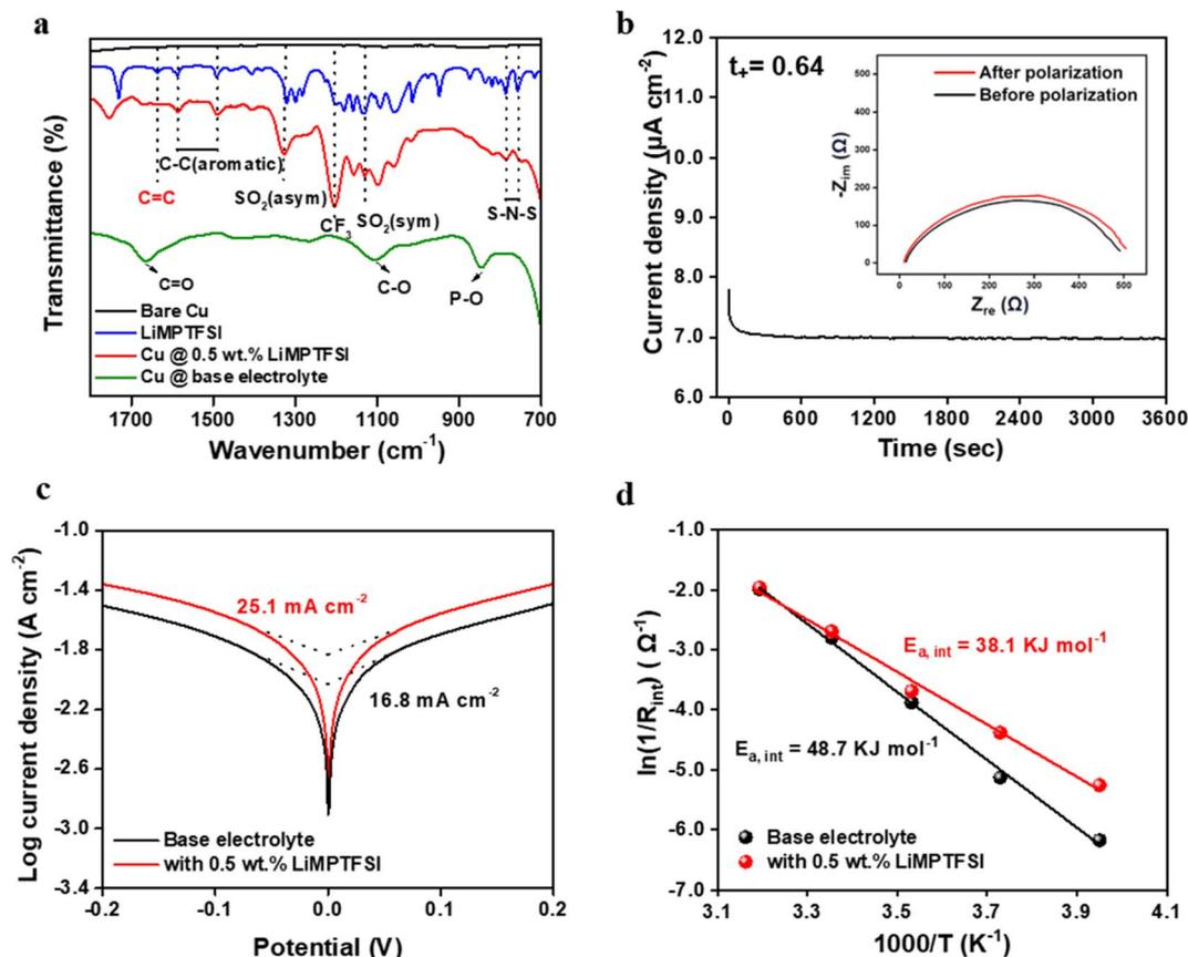
Fig. 2 (a) FT-IR spectra of bare Cu, LiMPtFSI powder, and surface modified Cu foils using the base electrolyte or electrolyte with 0.5 wt% LiMPtFSI. (b)  $t_+$  measurement and (c) Tafel plots of the surface modified Li symmetric cells using the base electrolyte with and without 0.5 wt% LiMPtFSI. (d) Temperature dependence of the interfacial resistance of the graphite anode after pre-cycling.
