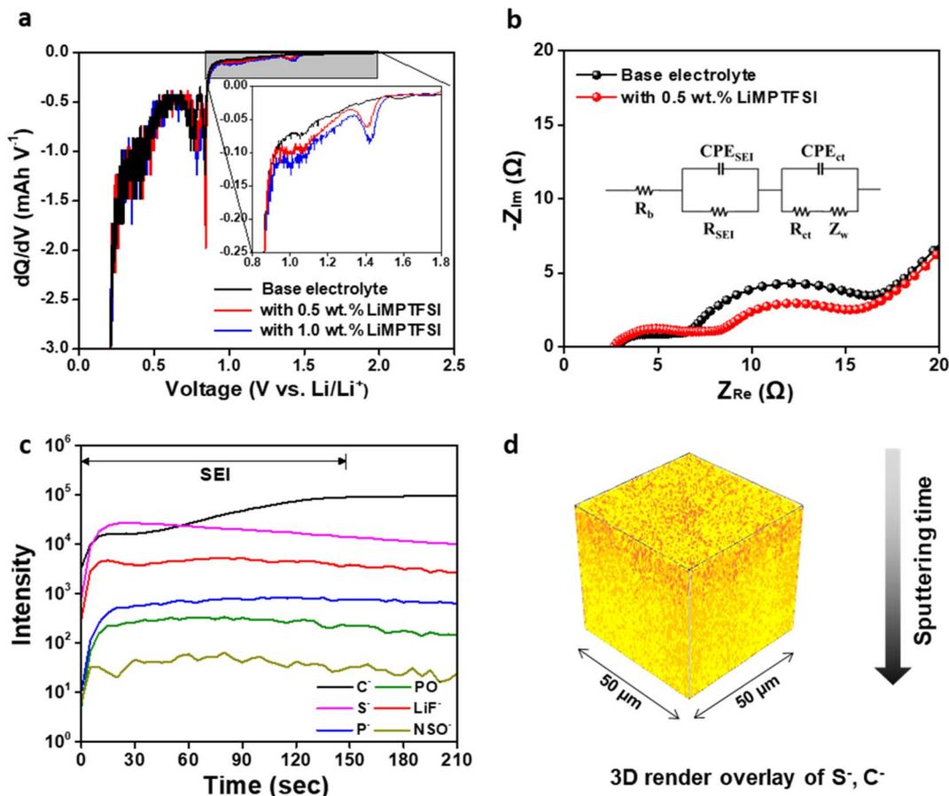
Fig. 3 (a)  $dQ/dV$  plot of the graphite electrodes containing different electrolytes. (b) Electrochemical impedance spectra of the Gr/NCM full cell after pre-cycling. (c) ToF-SIMS depth profile and (d) 3D rendered image of the graphite anode using the base electrolyte with 0.5 wt% LiMPTFSI after pre-cycling ( $S^-$ : orange,  $C^-$ : yellow).
