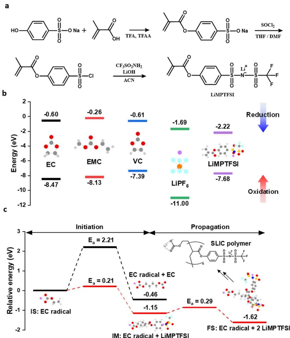
Fig. 1 (a) Synthetic route of LiMPTFSI. (b) HOMO and LUMO energy levels of EC, EMC, VC, LiPF<sub>6</sub> and LiMPTFSI. (c) Relative energies for dimerization of EC and LiMPTFSI by the EC radical. Initial state (IS): EC radical, intermediate state (IM): IS + LiMPTFSI, final state (FS): IM + LiMPTFSI.
