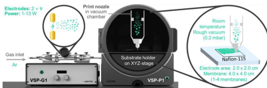
Figure 5 Schematic of the VSParticle nanoparticle printing technology. A certain wattage is applied to metal electrodes which causes the metal to ablate and particles to detach. The particles agglomerate to form nanoparticles as they are carried by inert Ar to a vacuum chamber where they are printed via a nozzle onto a substrate of choice held by an XYZ-stage. Reproduced with permission from ref. 110. Copyright 2022 MDPI.
