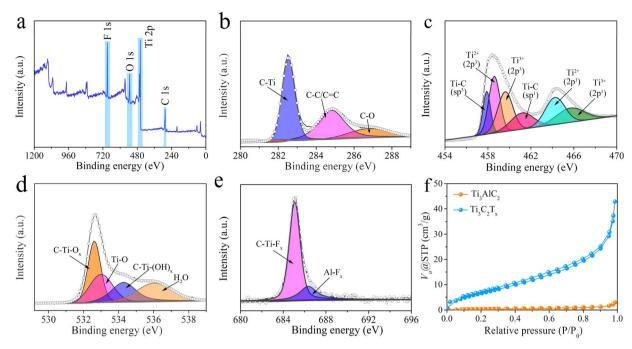
Fig. 3 (a) XPS survey spectrum of  $Ti_3C_2T_x$ . High resolution (b) C 1s, (c) Ti 2p, (d) O 1s, and (e) F 1s spectra of  $Ti_3C_2T_x$ . (f)  $N_2$  adsorption/desorption curves of  $Ti_3AlC_2$  and  $Ti_3C_2T_x$ .
