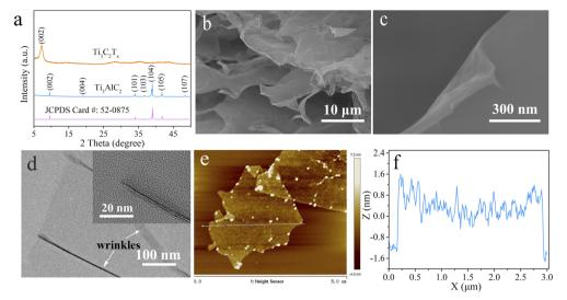
Fig. 2 (a) XRD plots of  $Ti_3AlC_2$  and  $Ti_3C_2T_x$  samples. (b and c) SEM images of the freeze-dried  $Ti_3C_2T_x$  MXene. (d) TEM image of  $Ti_3C_2T_x$  flakes. (e) The AFM image of  $Ti_3C_2T_x$  sheets. (f) The thickness curve of  $Ti_3C_2T_x$  sheets received from the AFM image.
