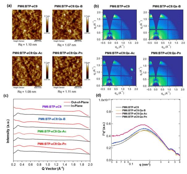
Fig. 3 (a) AFM height images and (b) 2D GIWAXS patterns of the BTP-eC9 binary and ternary blend films. (c) 1D GIWAXS line cuts of the BTP-eC9 binary and ternary blend films in the in-plane and out-of-plane directions. (d) Lorentz-corrected 1D R-SoXS profiles of the BTP-eC9 binary and ternary blend films.
