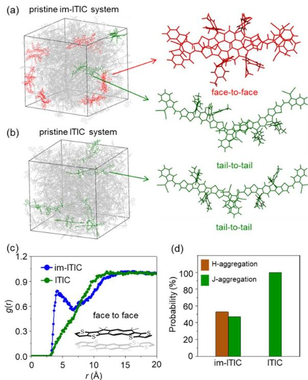
**Fig. 8** (a) and (b) Snapshots (left) and examples of stacking modes (right) from the MD results of im-ITIC and ITIC based pristine systems. (c) Radial distribution function data for pristine systems. (d) Probability of different aggregations in pristine systems. In the snapshots, face-to-face and tail-to-tail aggregations are colored red and green, respectively.
