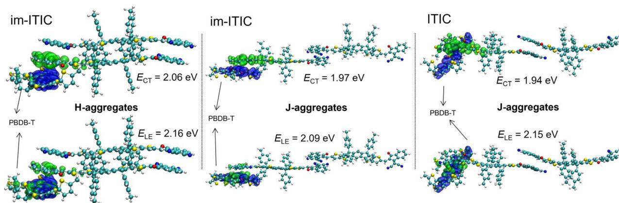
**Fig. 9** Distributions of the hole (blue) and electron (green) for different excited states of different aggregates of im-ITIC. TD-DFT calculations were performed using the  $\omega$ B97XD/6-31G(d,p) method on the molecular clusters from MD simulations.
