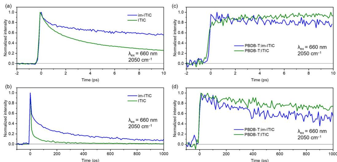
Fig. 7 Time profiles of free electrons in pristine **ITIC** and **im-ITIC** films (a & b) and in their blend films with PBDB-T (c & d). These profiles were obtained by photoexciting the NFA domain with a  $660\text{ nm}$  pump pulse and measuring the transient absorption at  $2050\text{ cm}^{-1}$ .
