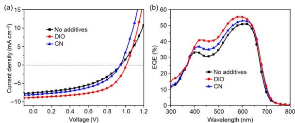
Fig. 5 (a)  $J$ - $V$  curves and (b) EQE spectra of PBDB-T:im-ITIC with different additives.
