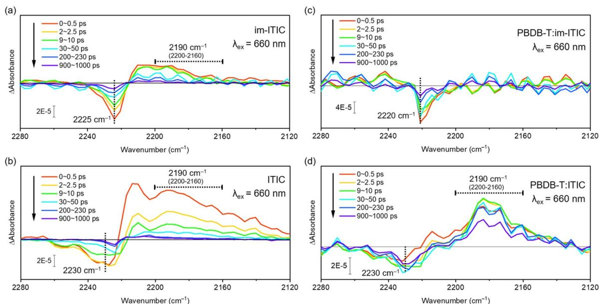
Fig. 6 Differential vibrational spectra of cyano groups in NFAs after pump pulse irradiation. Pristine (a) im-ITIC and (b) ITIC films are photoexcited by a 660 nm pump pulse. Additionally, the NFA domain in the blend film with PBDB-T is photoexcited by the same 660 nm pump pulse (panels c-d).
