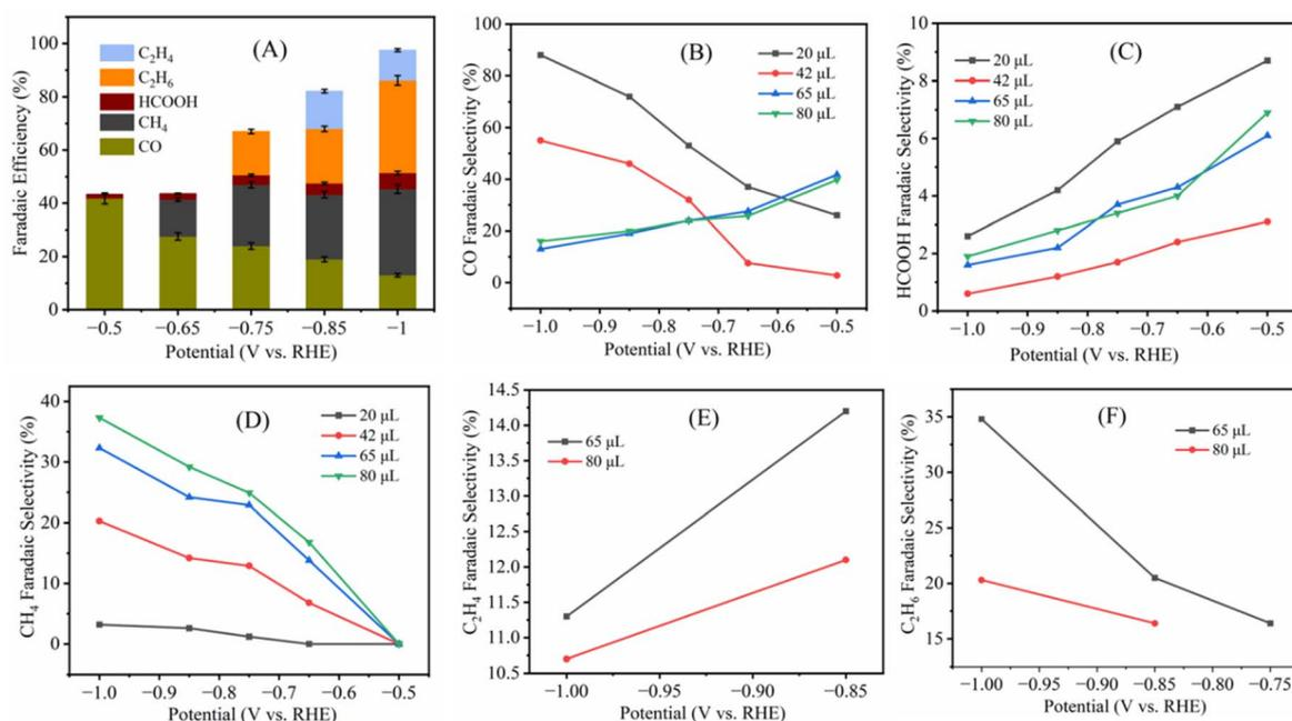
Fig. 1 Faradaic efficiency of different products ( $C_2H_4$ ,  $C_2H_6$ , HCOOH,  $CH_4$ , and CO) as a function of potential for the electrode CTC-65 during electrochemical reduction using a flow cell electrolyser (A); and faradaic selectivity of CO (B); HCOOH (C);  $CH_4$  (D);  $C_2H_4$  (E); and  $C_2H_6$  (F) as a function of potential for the electrodes loaded with different volumes of  $SnCl_4$  Lewis acid on the  $Cu_2O$  GDE.
