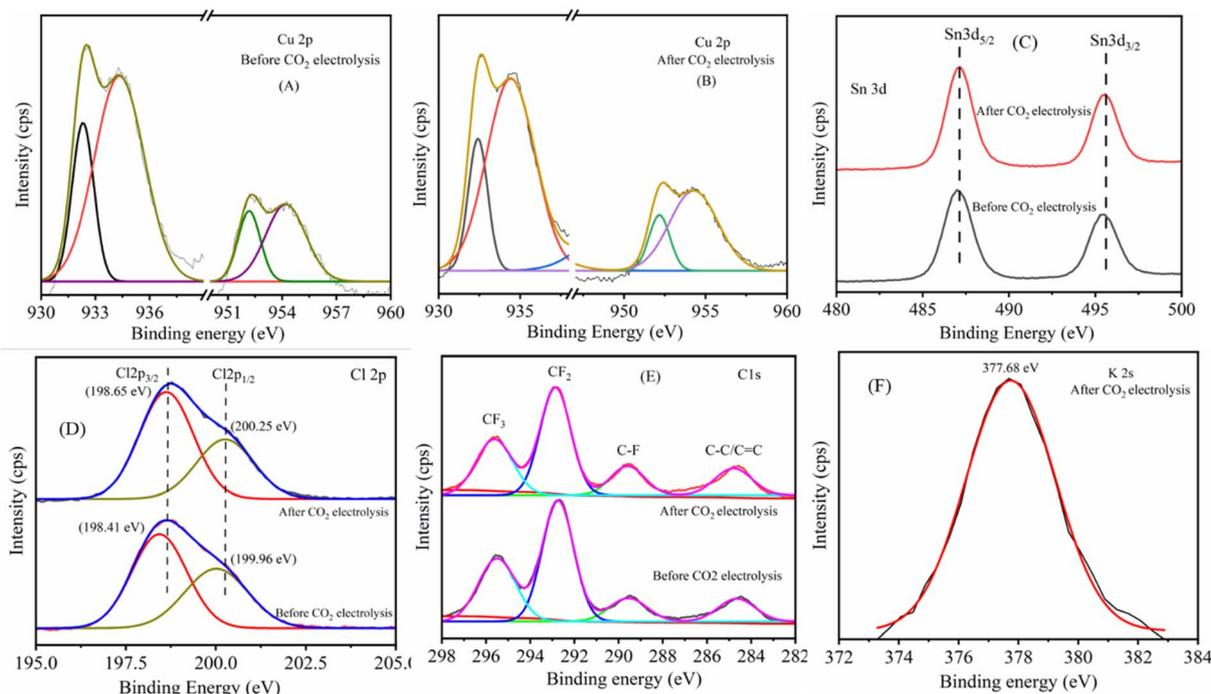
Fig. 5 XPS analysis of the CTC-65 electrode before and after CO<sub>2</sub> electrolysis, showing the spectra of Cu 2p (A and B), Sn 3d (C), Cl 2p (D), C 1s (E), and K 2s (F).
