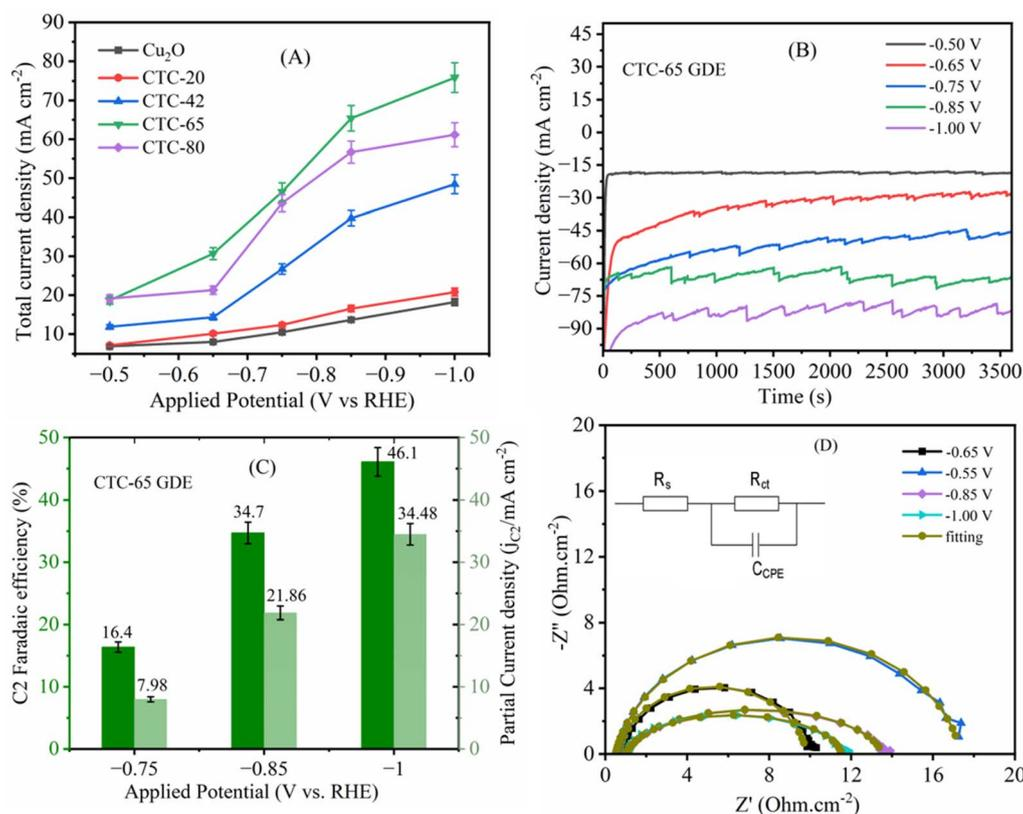
Fig. 7 (A) Total current density profiles for  $\text{Cu}_2\text{O}$ , CTC-20, CTC-42, CTC-65, and CTC-80 electrodes at various potentials; (B) constant potential electrolysis of CTC-65 at various potentials over 3600 seconds; (C) faradaic efficiencies of  $\text{C}_2$  products at various potentials with their corresponding partial current densities; and (D) electrochemical impedance spectra of the CTC-65 GDE at various potentials after  $\text{CO}_2$  electrolysis.
