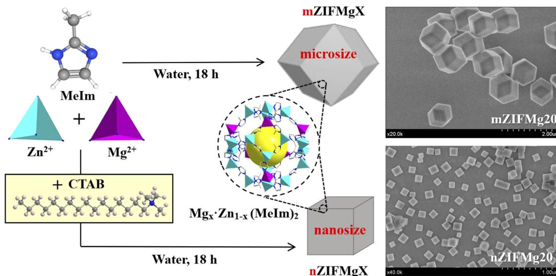
Fig. 1 Schematic illustration of the synthesis procedure of microsized mZIFMg<sub>x</sub> and nanosized nZIFMg<sub>x</sub> particles, including representative SEM images of the samples prepared with 20% mol Mg (nZIFMg<sub>20</sub> and mZIFMg<sub>20</sub>).
