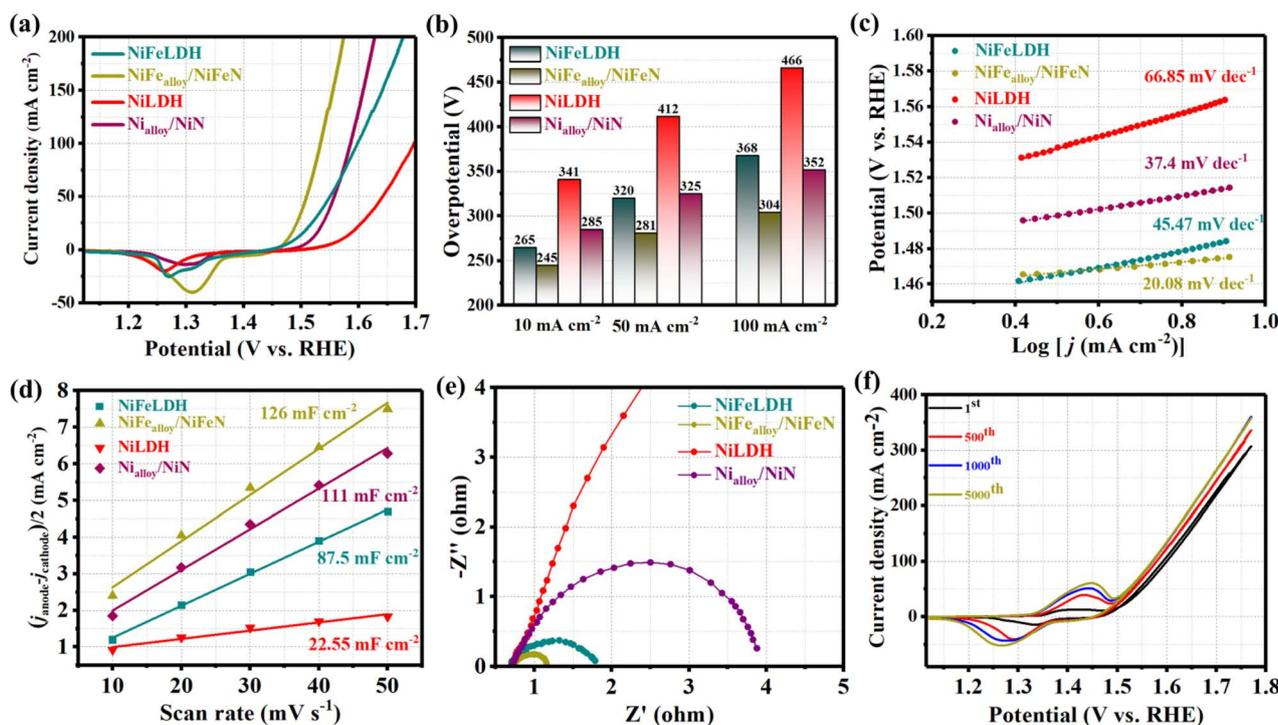
Fig. 4 Electrochemical measurement results of different samples in 1 M KOH: (a) LSV curves of OER; (b) overpotential histogram at 10, 50, and 100 mA cm<sup>-2</sup>; (c) Tafel plots; (d) capacitive current at 1.22 V vs. RHE as a function of the scan rate; (e) Nyquist plots measured at 0.6 V versus Hg/HgO; and (f) LSV curves of NiFe<sub>alloy</sub>/NiFeN before and after multiple CV cycles.
