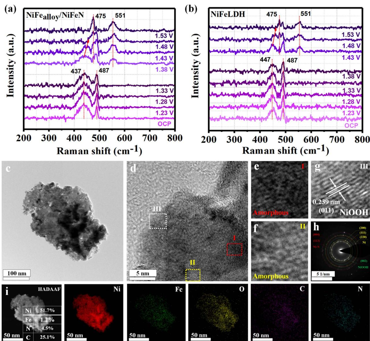
Fig. 6 *In situ* Raman spectra of (a) NiFe<sub>alloy</sub>/NiFeN and (b) NiFeLDH under various applied potentials (*vs.* RHE). Morphology and structure characterization of NiFe<sub>alloy</sub>/NiFeN after OER: (c) TEM image; (d) HRTEM image. (e–g) Atomic lattice image of the three selected dashed areas in (d). (h) SAED pattern and (i) HADAAAF image and EDX spectra with the main metal element mappings.
