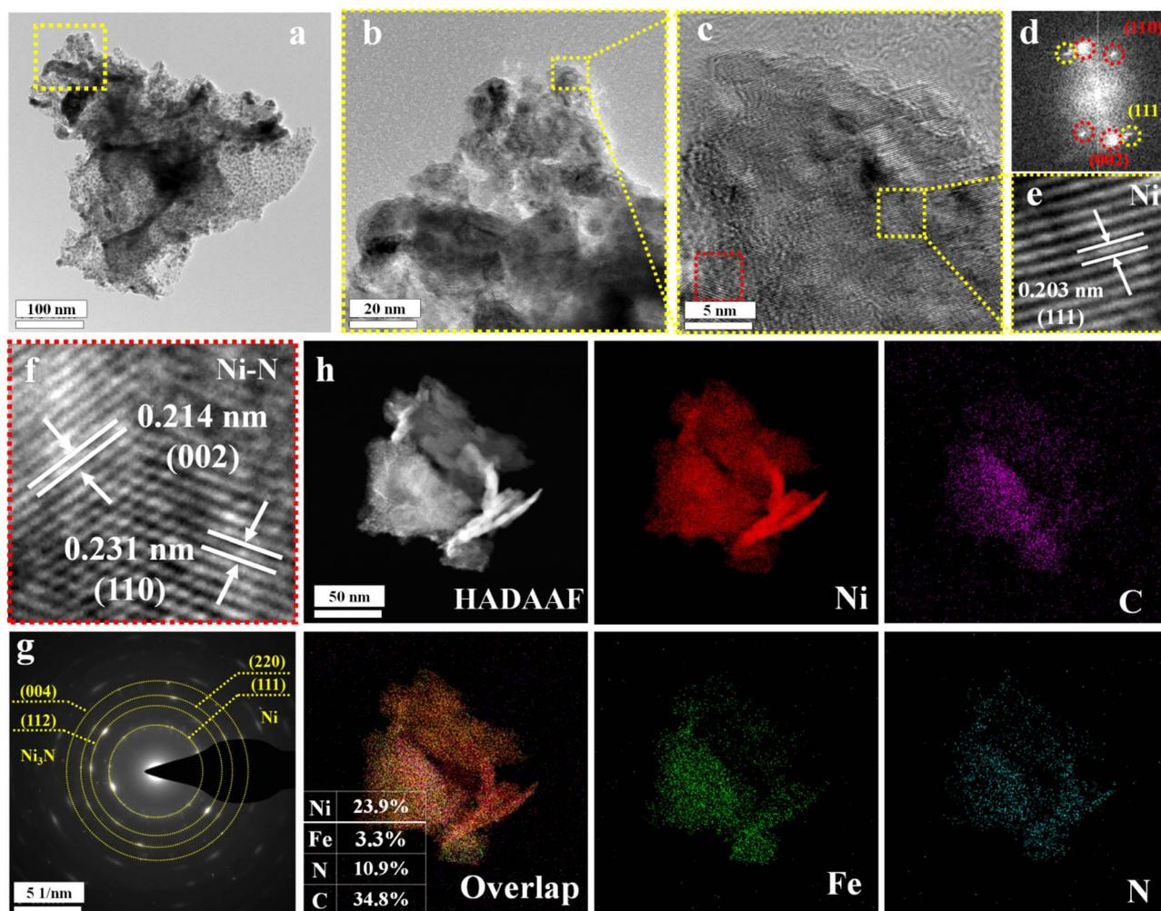
Fig. 2 Morphology and structure characterization of NiFe<sub>alloy</sub>/NiFeN: (a and b) TEM images; (c) HRTEM image; and (d) FFT image of the surface; (e) atomic lattice image of Ni alloy of the yellow dashed area in (c); (f) atomic lattice image of Ni–N of the red dashed area in (c); (g) SAED pattern; (h) HADAAE image and EDX spectra with the main metal element mappings.
