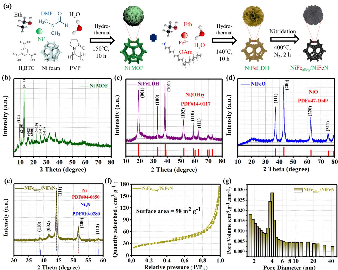
Fig. 1 (a) Schematic illustrating the construction of NiFe<sub>alloy</sub>/NiFeN as a pre-catalyst; phase and bonding structure of the materials under study; XRD patterns of (b) Ni MOF; (c) NiFeLDH; (d) NiFeO; and (e) NiFe<sub>alloy</sub>/NiFeN; (f) N<sub>2</sub> adsorption–desorption isotherms of NiFe<sub>alloy</sub>/NiFeN; and (g) pore size distribution curves of NiFe<sub>alloy</sub>/NiFeN.
