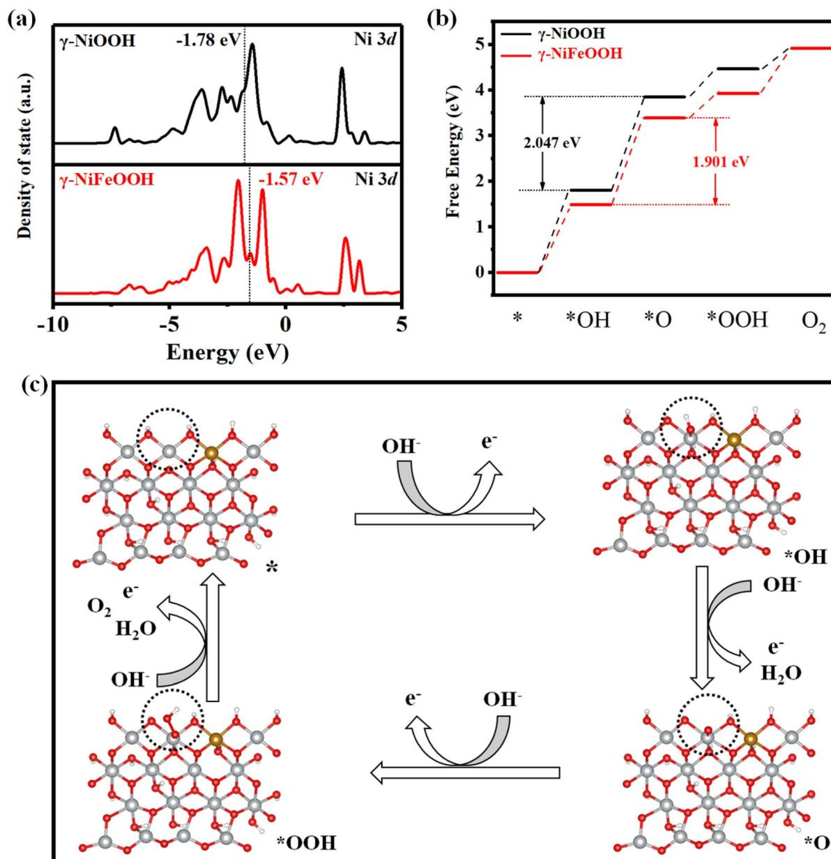
Fig. 8 (a) DOS of  $\gamma$ -NiFeOOH and  $\gamma$ -NiOOH with respect to the Ni 3d orbital. (b) Calculated Gibbs free energy diagram of  $\gamma$ -NiFeOOH and  $\gamma$ -NiOOH over the four steps of the OER process. (c) Adsorbate evolution mechanism (AEM) of the  $\gamma$ -NiFeOOH OER catalytic process.
