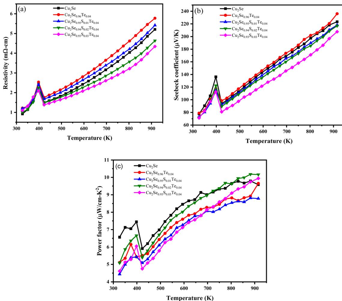
Fig. 4 (a) Electrical resistivity; (b) thermopower; (c) power factor for  $\text{Cu}_2\text{Se}$  and  $\text{Cu}_2\text{Se}_{0.96-x}\text{S}_x\text{Te}_{0.04}$  ( $x = 0.00, 0.01, 0.02, \text{ and } 0.03$ ) sintered at 923 K for 6 h in vacuum.
