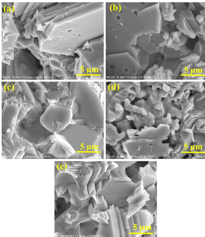
**Fig. 3** FE-SEM of (a)  $\text{Cu}_2\text{Se}$ , (b)  $\text{Cu}_2\text{Se}_{0.96}\text{Te}_{0.04}$ , (c)  $\text{Cu}_2\text{Se}_{0.95}\text{S}_{0.01}\text{Te}_{0.04}$ , (d)  $\text{Cu}_2\text{Se}_{0.94}\text{S}_{0.02}\text{Te}_{0.04}$ , (e)  $\text{Cu}_2\text{Se}_{0.93}\text{S}_{0.03}\text{Te}_{0.04}$ .
