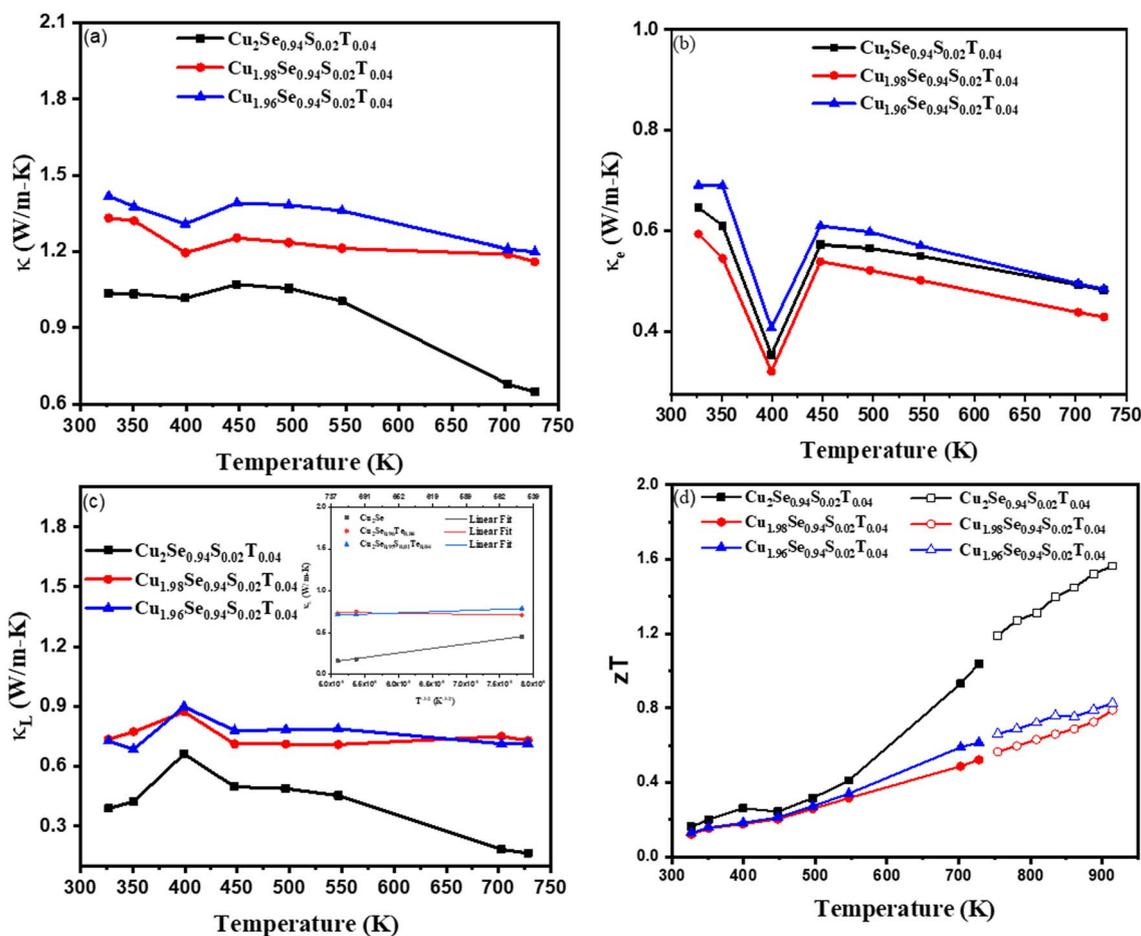
Fig. 8 (a) Total thermal conductivity ( $\kappa$ ); (b) electronic thermal conductivity ( $\kappa_e$ ); (c) lattice thermal conductivity ( $\kappa_L$ ) and inset with  $\kappa_L \sim T^{-3/2}$ ; (d) zT for Cu<sub>2-y</sub>Se<sub>0.94</sub>S<sub>0.02</sub>Te<sub>0.04</sub> ( $y = 0.00, 0.02, \text{ and } 0.04$ ) sintered at 923 K for 6 h in vacuum.
