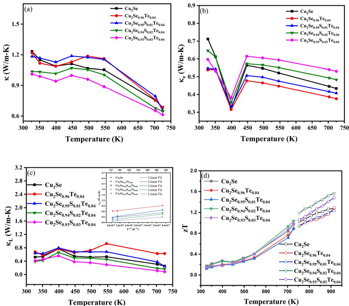
Fig. 5 (a) Total thermal conductivity ( $\kappa$ ); (b) electronic thermal conductivity ( $\kappa_e$ ); (c) lattice thermal conductivity ( $\kappa_L$ ) and inset the fig  $\kappa_L \sim T^{-3/2}$ ; (d)  $zT$  for Cu<sub>2</sub>Se and Cu<sub>2</sub>Se<sub>0.96-x</sub>S<sub>x</sub>Te<sub>0.04</sub> ( $x = 0, 0.01, 0.02, \text{ and } 0.03$ ) sintered at 923 K for 6 h in vacuum.
