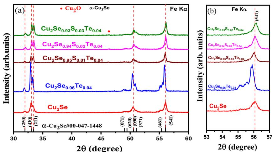
Fig. 2 XRD patterns of Cu<sub>2</sub>Se and Cu<sub>2</sub>Se<sub>0.96-*x*</sub>S<sub>*x*</sub>Te<sub>0.04</sub> (*x* = 0.00, 0.01, 0.02, and 0.03): (a) samples sintered at 923 K for 6 h under vacuum, and (b) magnified view for detailed analysis.
