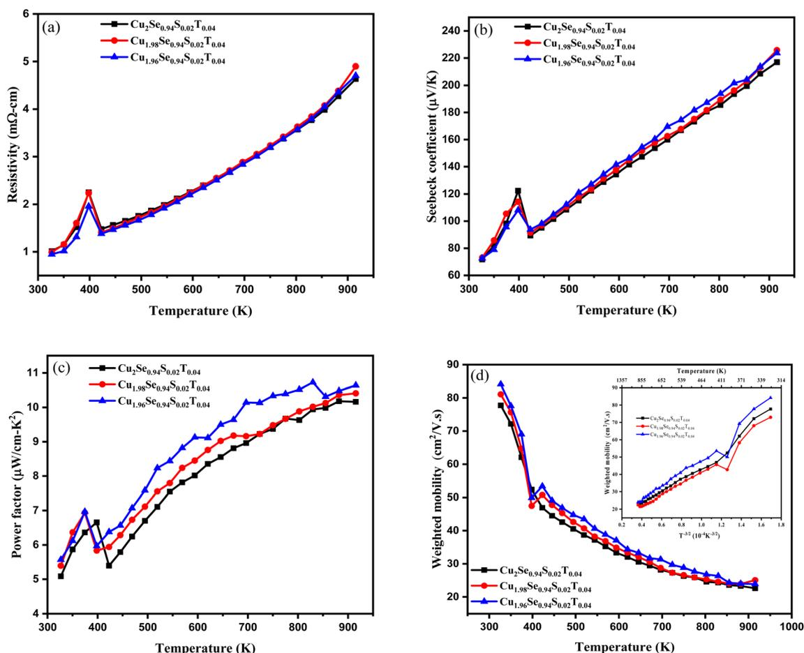
Fig. 7 (a) Electrical resistivity; (b) thermopower; (c) power factor; (d) weighted mobility and inset weighted mobility vs.  $T^{3/2}$  for  $\text{Cu}_{2-y}\text{Se}_{0.94}\text{S}_{0.02}\text{Te}_{0.04}$  ( $y = 0.00, 0.02, \text{ and } 0.04$ ) sintered at 923 K for 6 h in vacuum.
