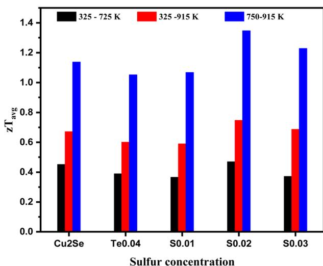
Fig. 6 Average  $zT$  ( $zT_{\text{avg}}$ ) for  $\text{Cu}_2\text{Se}$  and  $\text{Cu}_2\text{Se}_{0.96-x}\text{S}_x\text{Te}_{0.04}$  ( $x = 0.00, 0.01, 0.02,$  and  $0.03$ ) sintered at 923 K for 6 h in vacuum.
