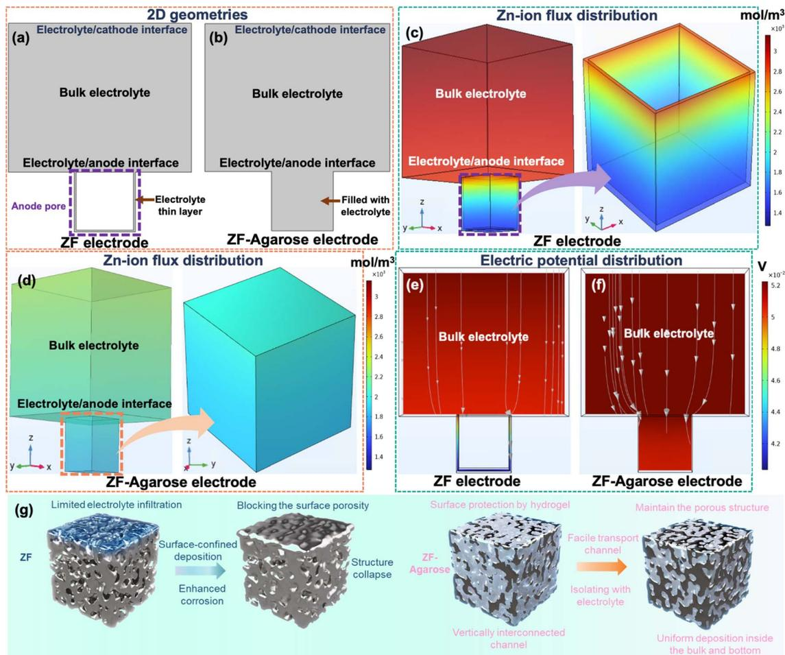
Fig. 4 The COMSOL simulation of ion flux and electric field distribution and schematic representation of deposition regimes. The basic 2D simulation model for (a) ZF and (b) ZF-agarose electrodes. The Zn-ion flux distribution of (c) ZF and (d) ZF-agarose electrode. The electric potential distribution of (e) ZF and (f) ZF-agarose electrodes. (g) Schematic diagram of ZF and ZF-agarose electrode for illustration of different Zn-deposition manners.
