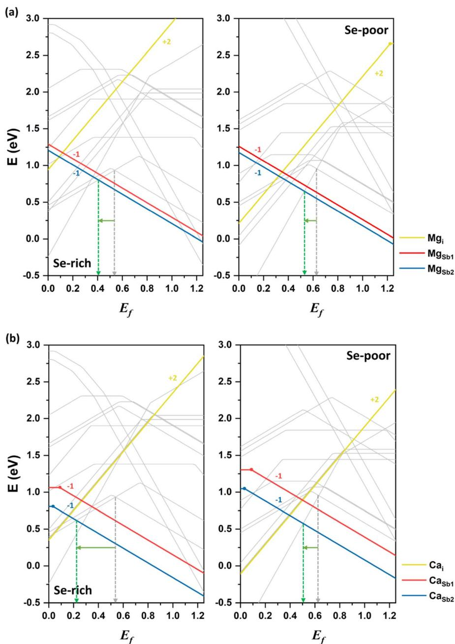
Fig. 7 Formation energies of alkaline earth dopants, (a) Mg and (b) Ca, in  $\text{Sb}_2\text{Se}_3$  under Se-rich (left) and Se-poor (right) conditions as a function of the Fermi level ( $E_f$ ) compared with the formation energies of the intrinsic defects represented by gray lines. The dashed gray and green arrows indicate the Fermi levels expected in the undoped and doped systems, respectively.
