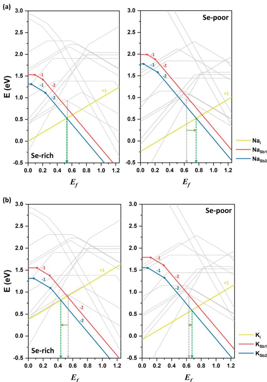
Fig. 6 Formation energies of alkali dopants, (a) Na and (b) K, in  $\text{Sb}_2\text{Se}_3$  under Se-rich (left) and Se-poor (right) conditions as a function of the Fermi level ( $E_f$ ) compared with the formation energies of the intrinsic defects represented by gray lines. The dashed gray and green arrows indicate the Fermi levels expected in the undoped and doped systems, respectively.
