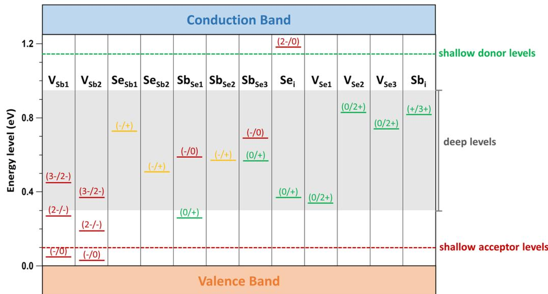
Fig. 4 Calculated transition energy levels of intrinsic defects within the bandgap of  $\text{Sb}_2\text{Se}_3$ . Red, green, and yellow bars represent acceptor, donor, and amphoteric defect levels, respectively. The dashed red and green lines, along with the gray box, indicate ionization levels within the bandgap, distinguishing shallow defect levels from deep defect levels.
