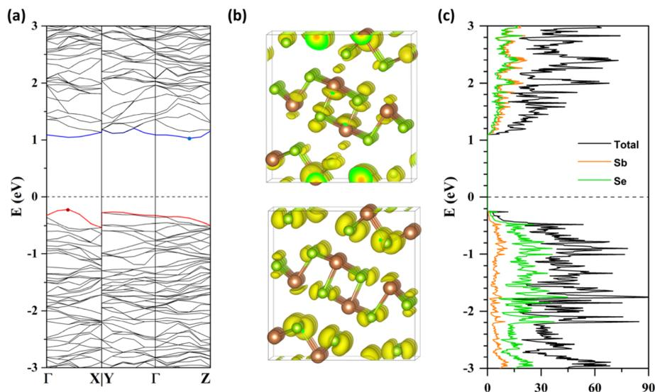
Fig. 2 (a) Band structure, (b) partial charge densities of the CBM (top) and VBM (bottom), and (c) DOS of the  $\text{Sb}_2\text{Se}_3$  supercell. In panel (a), the red and blue lines represent the VBM and CBM, respectively, with the Fermi level shifted to zero.
