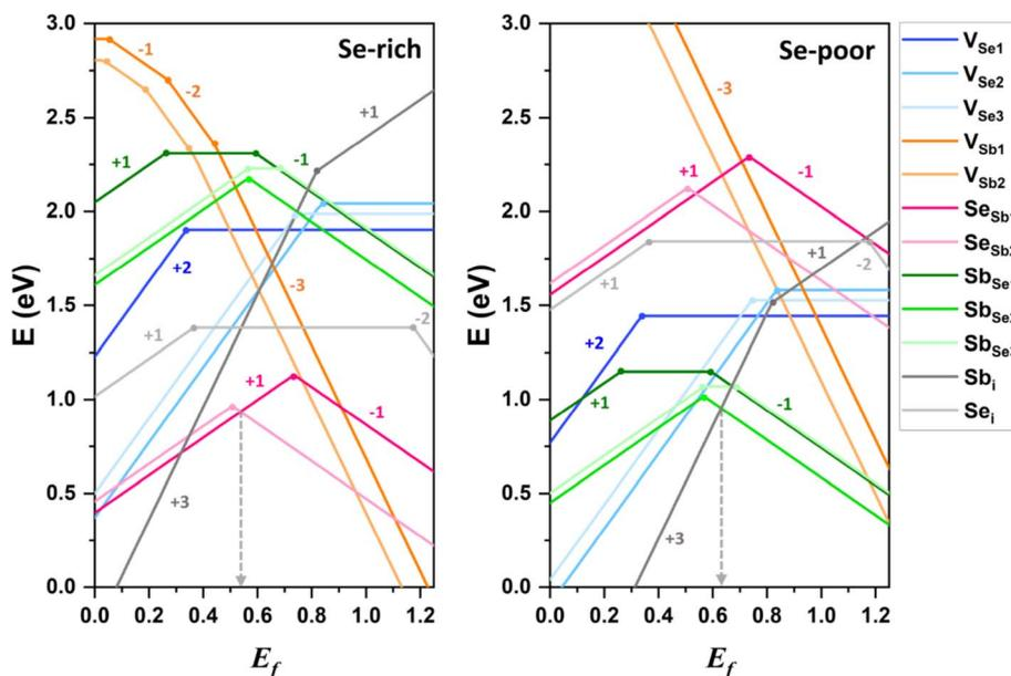
Fig. 3 Formation energies of intrinsic defects in  $\text{Sb}_2\text{Se}_3$  under Se-rich (left) and Se-poor (right) conditions as a function of the Fermi level ( $E_f$ ). The dashed grey arrow indicates the Fermi level expected in  $\text{Sb}_2\text{Se}_3$ .
