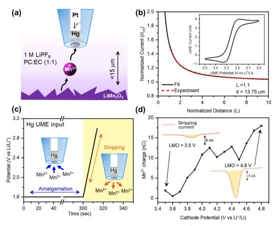
Fig. 2 In situ Mn detection in the SECM configuration. (a) Depiction of the SECM setup for  $Mn^{2+}$  detection with the Hg UME and LMO cathode in 1 M LiPF<sub>6</sub> PC: EC (1:1) electrolyte. (b) Probe approach curve using TCNQ as a redox mediator. The CV of TCNQ is depicted in the inset. (c) The potential input at the Hg UME for ASV measurement. (d) Representative final output of the SECM experiment, obtained by integrating the area under the curve of the Hg UME stripping current.
