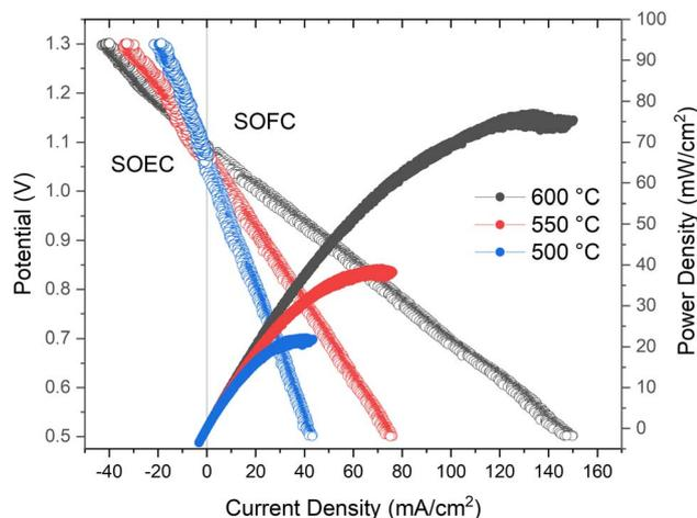
Fig. 8  $j$ - $V$  and  $j$ - $P$  curves of electrolyte-supported cell at different temperatures measured under dry synthetic air and humidified (3%  $\text{H}_2\text{O}$ ) hydrogen flows in SOFC and SOEC modes.
