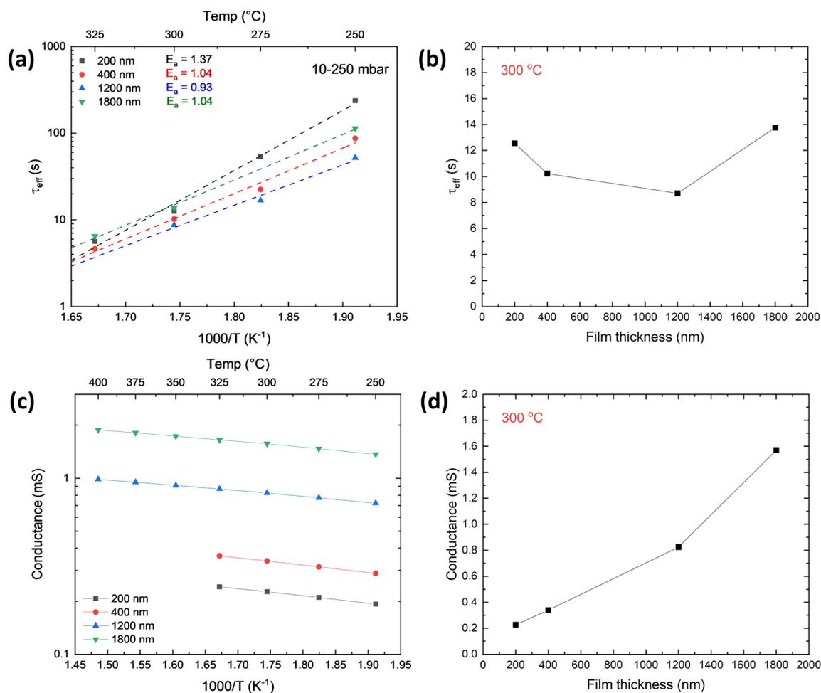
Fig. 3 (a) Arrhenius plot of the effective time constant ( $\tau_{\text{eff}}$ ) obtained from ECR measurements during a  $p\text{O}_2$  change from 10 to 250 mbar, and (b) comparison of the  $\tau_{\text{eff}}$  at different film thickness at 300 °C; (c) Arrhenius plot of the electrical conductance measured using the van der Pauw configuration at a  $p\text{O}_2$  of 250 mbar between 250–400 °C, and (d) comparison of the conductance of films with different thickness at 300 °C.
