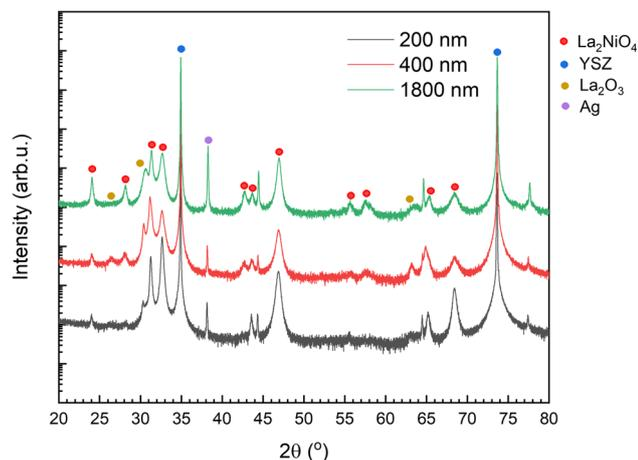
Fig. 2 XRD spectra of L2NO4 thin films of various thicknesses (200, 400 and 1800 nm) grown on a YSZ single-crystal substrate.
