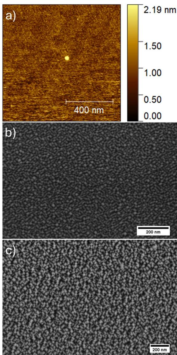
**Fig. 4** Microstructural characterization of as deposited NiCGO-based thin films showing (a) AFM micrograph of dense NiCGO<sub>5mT-700C</sub>; (b) SEM micrographs for the rest of the NiCGO thin films fabricated: NiCGO<sub>150mT-700C</sub>, and (c) NiCGO<sub>200mT-500C-TT</sub>.
