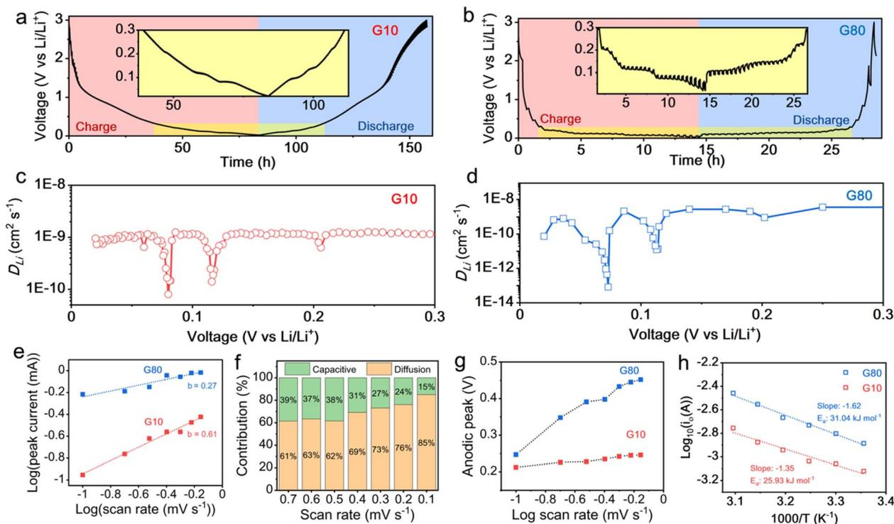
Fig. 5 Kinetic analysis of G10 and G80. (a) and (b) GITT profiles of G10 and G80, respectively. (c) and (d)  $D_{Li}$  of G10 and G80 during the charge process. (e) The  $b$  value is the slope function of the log scan rate ( $v$ ) vs. log peak current ( $i$ ) for G10 and G80. (f) Capacitive and diffusion contribution ratios for G10 at different scan rates. (g) Anodic peak shifts of G10 and G80 at various scan rates. (h)  $\log i_0$  vs.  $1000/T$  plot of G10 and G80.
