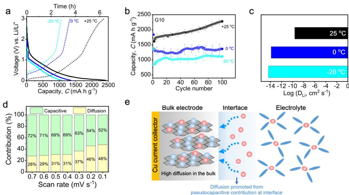
Fig. 6 Low-temperature performance of G10. (a) and (b) Galvanostatic and capacity profiles at various temperature ranges. (c)  $D_{\text{Li}}$  at different temperatures. (d) Capacitive and diffusion contribution ratio at sub-zero temperature (–20 °C). (e) Schematic illustration of the lithiation process of G10 at low temperatures.
