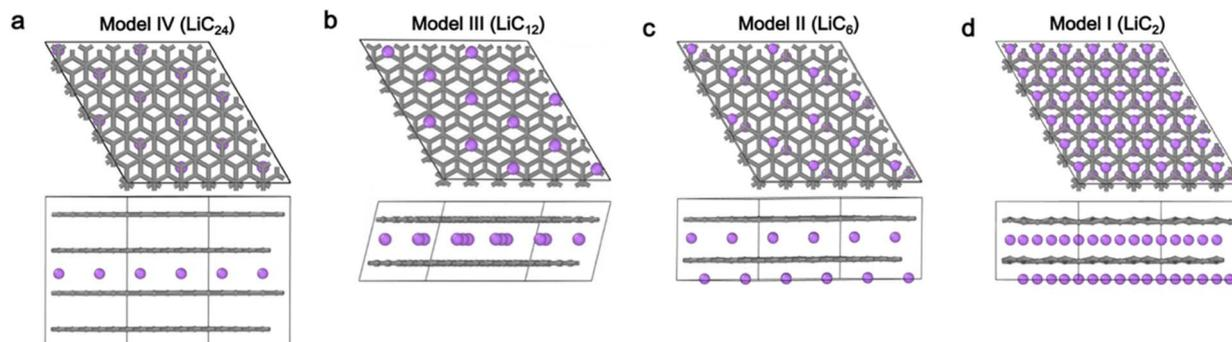
Fig. 4  $\text{Li}^+$  intercalation models. Top/side views of (a) Model IV ( $\text{LiC}_{24}$ ), (b) Model III ( $\text{LiC}_{12}$ ), (c) Model II ( $\text{LiC}_6$ ) and (d) Model I ( $\text{LiC}_2$ ).
